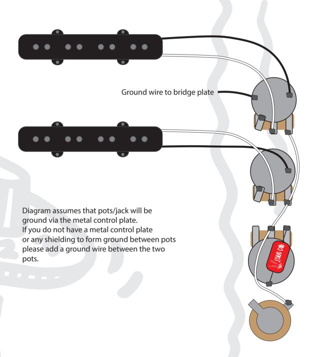
This diagram has been drawn with traditional 2 conductor braided pickup wires in mind. If your pickup is different to this, then please refer to that manufacturer's wire colour coding prior to installing.
