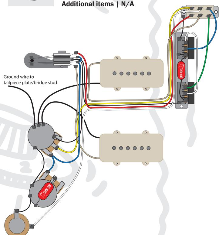
This diagram has been drawn with traditional 2 conductor pickup wires in mind. If your pickups are wired differently to this, then please refer to that manufacturer's wire colour coding prior to installing.
