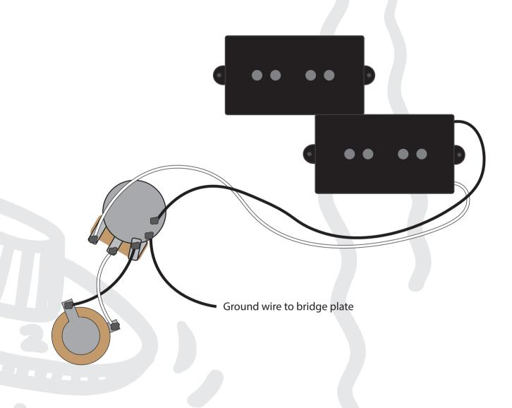
This diagram has been drawn with traditional 2 conductor braided pickup wires in mind. If your pickup is different to this, then please refer to that manufacturer's wire colour coding prior to installing.
