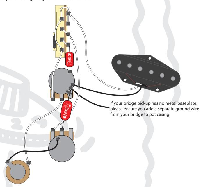
This diagram has been drawn with traditional 2 conductor pickup wires in mind. If your pickup is different to this, then please refer to that manufacturer's wire colour coding prior to installing.
