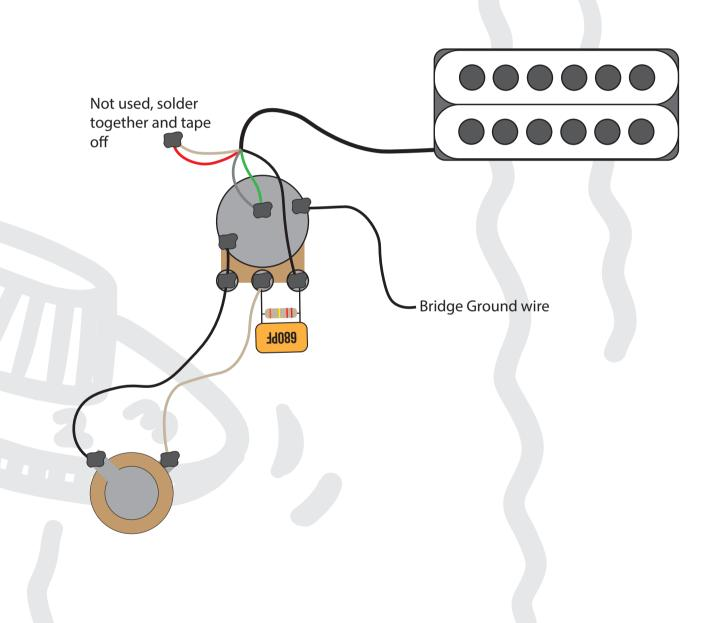
This diagram has been drawn with the Seymour Duncan Invader pickup wire colour codes in mind. If your pickup is different to this, or importantly, a different pickup manufacturer, then please refer to that manufacturer's wire colour coding prior to installing.
