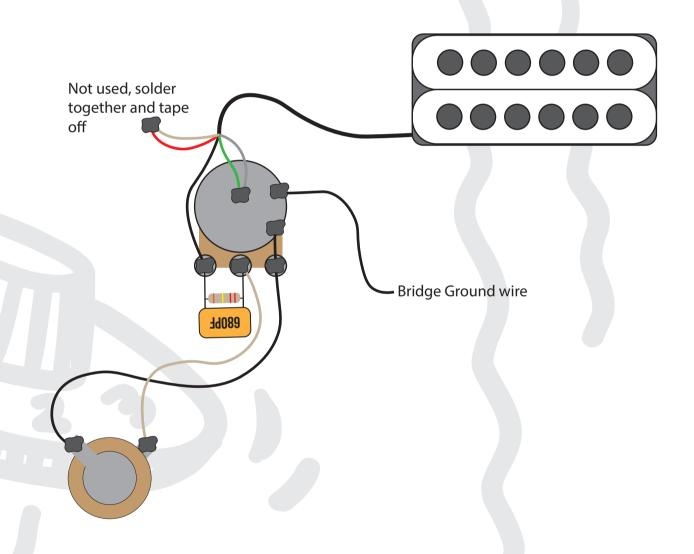
This diagram has been drawn with the Seymour Duncan Invader pickup wire colour codes in mind. If your pickup is different to this, or importantly, a different pickup manufacturer, then please refer to that manufacturer's wire colour coding prior to installing.
