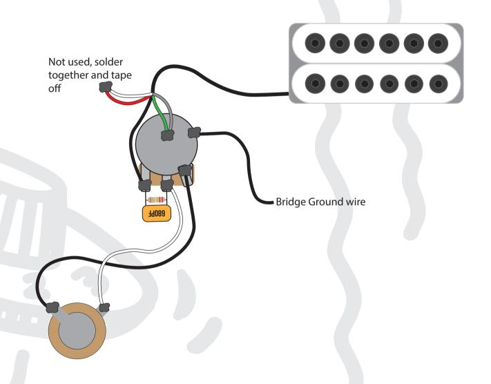
This diagram has been drawn with the Seymour Duncan 4 conductor pickup wire colour codes in mind. If your pickup is different to this, or importantly, a different pickup manufacturer, then please refer to that manufacturer's wire colour coding prior to installing.
