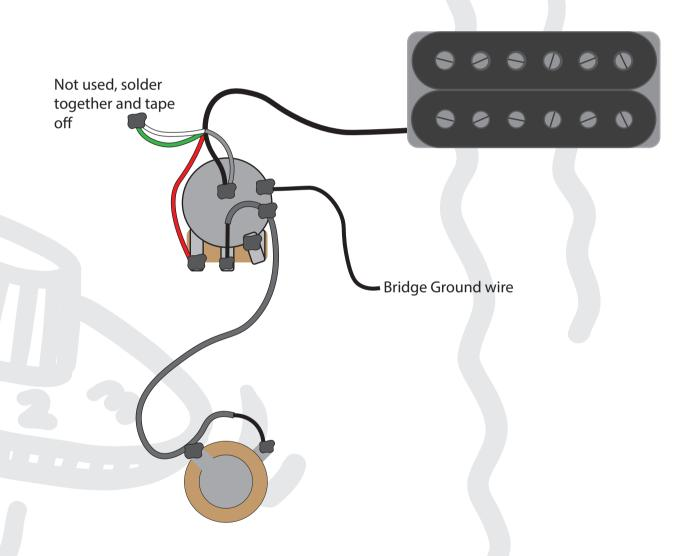
This diagram has been drawn with the Gibson 'Dirty Fingers' 4 conductor pickup wire colour codes in mind. If your pickup is different to this, or importantly, a different pickup manufacturer, then please refer to that manufacturer's wire colour coding prior to installing.
