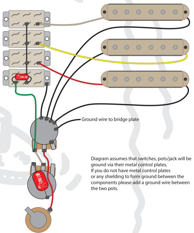
This diagram has been drawn with traditional 2 conductor braided pickup wires in mind. If your pickup is different to this, then please refer to that manufacturer's wire colour coding prior to installing.
