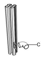
Place the 90° Rail Connector on the Rail Connector Clamp.
