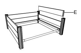
Use the 152 x 22mm Panel - L to assemble the three side panels of the Whelping Box.
