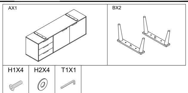
Please do not tight any bolt unless all bolts are fixed at their respective places. After fixing the bolts tighten them simultaneously. Note: 1.
