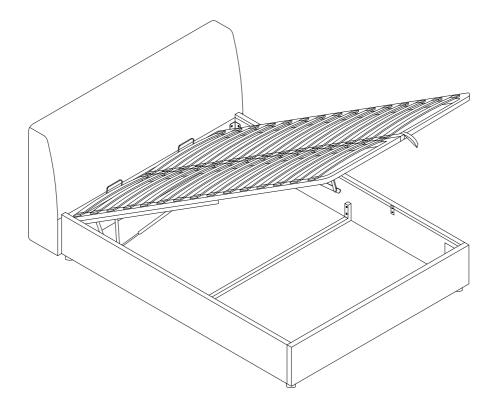
REMARK: FINALLY, PLACE MATTRESS ON FRAME THEN SLOWLY PUSH DOWN METAL FRAME ENSURING THE FRAME IS FULLY ALIGNED WITH THE SIDE RAIL.
