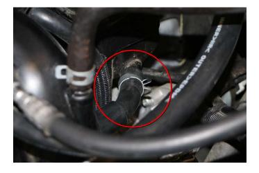
**b.** Use a Phillips screwdriver to remove the screw on the manifold tab.
