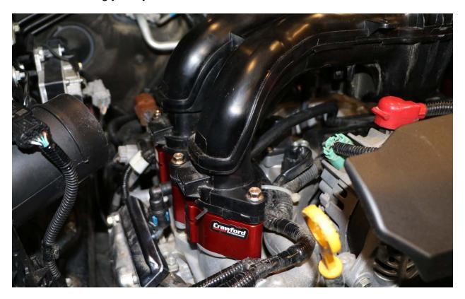
**b.** Place each block gasket side down on to the heads, matching up the marked position with the corresponding head.
