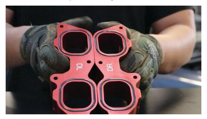
**9.** While lifting up the Intake Manifold, rotate EGR Pipe 180° to release it, and pull out. This part will not be reinstalled, but we recommend storing it in case you need to later revert your vehicle back to stock. Make sure the gasket pictured below stays in place.
