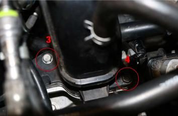
b. Remove 4 bolts from Driver's RH Side
