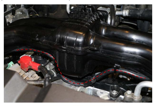
7. Remove the PCV hose marked below by pulling it off. This part will not be reinstalled, but we recommend storing it in case you need to later revert your vehicle back to stock.
