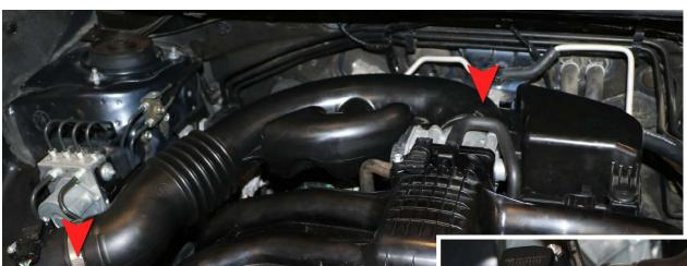
**c.** Use a flathead screwdriver to loosen the 2 worm clamps.
