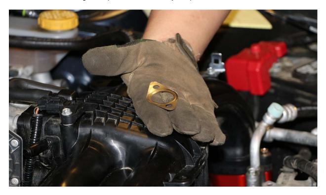
**10.** Lift up manifold and place blocks, with the fuel lines running between the 2 openings in the block. Be sure to do this step quickly and preferably in a clean environment as to avoid any contaminants entering your cylinder heads.
