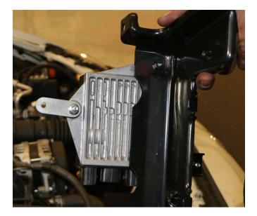
\*\*VERY IMPORTANT: This bracket MUST be installed in order to ground the Injector Control Unit. Without it, your vehicle will not be operational.
