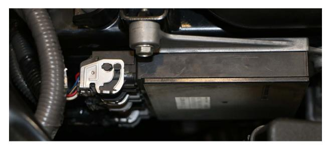
For the first plug, push in tab and rotate silver cover open. For the 2nd, rotate plastic cover open.
