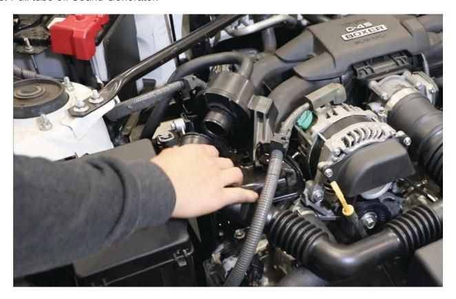
**d.** Locate and disconnect 4 plugs from the Injector Control Unit, pictured below. Each plug has a unique way to release.
