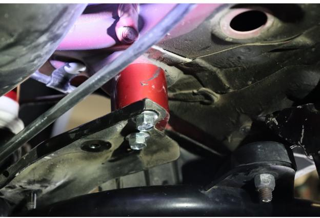
16. Install the hand brake bracket spacer using the provided M8X1.25X60 MM bolt. Push the 60 MM bolt through the underside of the sub frame support bracket as shown and place the provided spacer over the bolt. Fasten the brake line bracket to the top of the 60 MM bolt with the provided 12 MM nut. Torque to 25 ft-lbs. Repeat for the opposite side. (12 MM Socket and Wrench)
