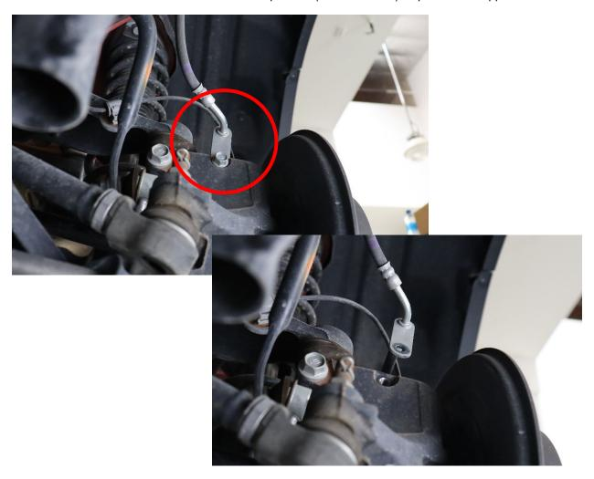
**5.** Remove the two bolts shown below from the sub-frame bracket. (14 MM Socket) Repeat for the opposite side.
