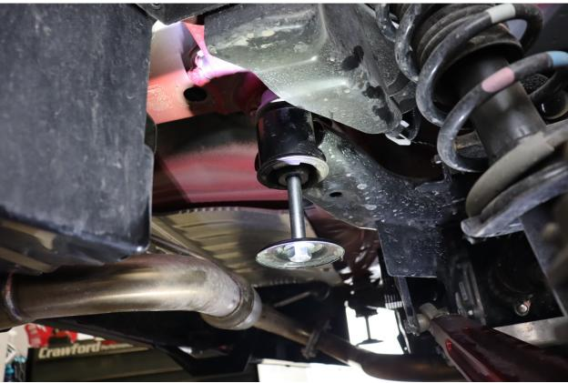
10. Go back to the rear sub-frame bolt first removed in step 8. Partially remove the 200 MM bolt from the sub-frame to allow room for the sub-frame spacer to fit between the chassis and the body of the vehicle. (19 MM Socket) Once the spacer is in position, tighten the 200 MM bolt into the subframe. Do not torque yet.
