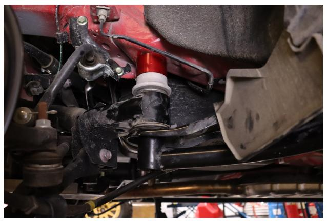
**14.** Install the sub-frame support spacer. This will be placed between the sub-frame support bracket where the bolts from step 5 were removed. Use the provided M10X1.25X60 MM bolts to ensure enough thread length for the spacer. **Torque to 25 ft-lbs**. (14 MM Socket)
