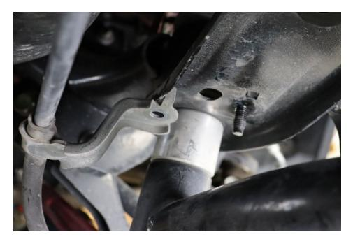
4. Remove the rear brake line bracket on the rear spindles. (10 MM Socket) Repeat for the opposite side.
