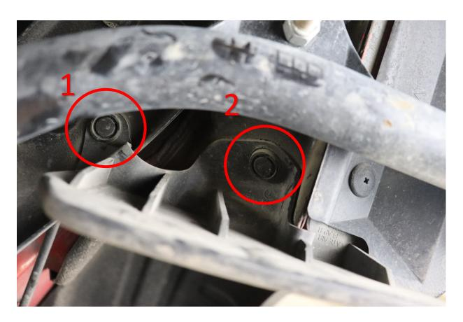
3. Remove the hand brake cable bracket. (10 MM Socket) Repeat for other side.
