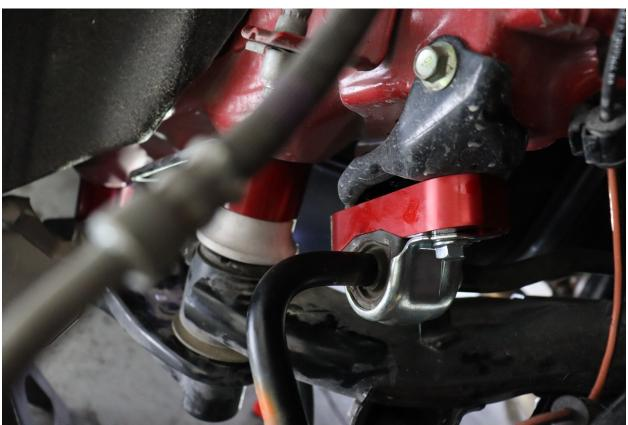
**20.** Reinstall the brake line bracket with the provided extension and 10 MM hardware. Place the extension bracket onto the spindle using the OEM hardware removed in step 4. **Torque both points to 18 ft-lbs**.
