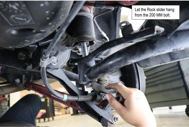
8. With the jack stand supporting the differential, locate and remove the first sub-frame bolt. (19 MM Socket) REMOVE AND REPLACE THE REAR SUB-FRAME BOLTS ONE AT A TIME. This is done to avoid getting the body and the subframe out of alignment
