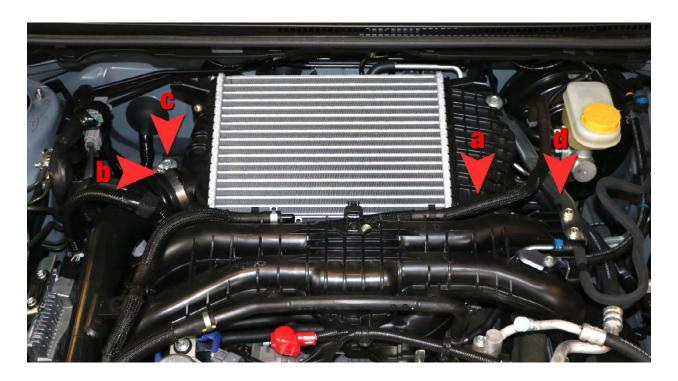
a. Loosen the throttle body clamp using a flathead screwdriver or 8mm socket and ratchet.
