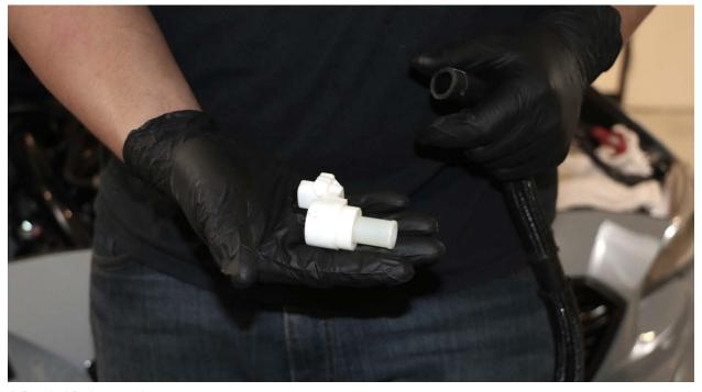
**11.** Slip a supplied worm clamp over one end of the supplied 52" 5/8" Vent Hose, then push hose onto the white connector. A thin layer of grease/lube will make this easier. Tighten clamp using a flathead screwdriver or 7mm socket and ratchet.
