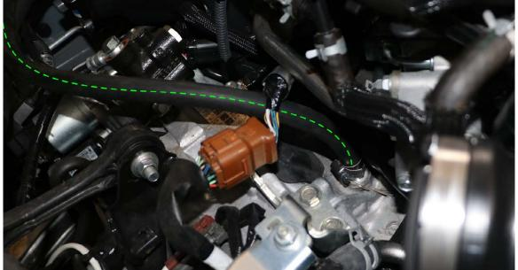
Connect the other end of the hose to port #4 on the AOS. Slip over a supplied worm clamp, push the hose on to the port, then position and tighten the worm clamp with a flathead screwdriver or 7mm ratchet and socket.
