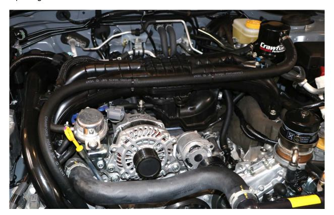
**14.** Remove PCV Hose behind the intake manifold. Using pliers, open the clamps while moving them away from the ends of the hose. Pull off.
