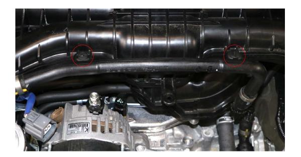
**b.** Disconnect plastic fitting on PCV hose connector. This can be done without breaking the fitting. Use slip joint pliers to squeeze the round fitting at it's largest diameter, just above the joint, until you hear an audible click, then use a flathead to pry open the fitting at it's joint.
