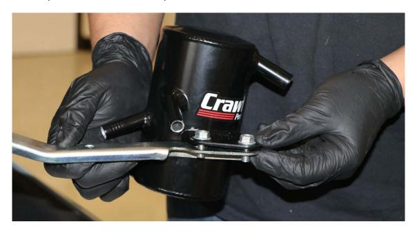
**b.** Tighten 2 bolts using a 12mm socket and ratchet.
