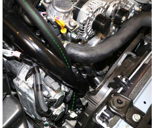
**13.** Run the hose along the same path as the OEM hose; along the front of the intake manifold. Use zip ties to secure the hose to the pin brackets.
