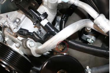
**g.** Lift up AC compressor and set on battery with some rags laid down for protection.
