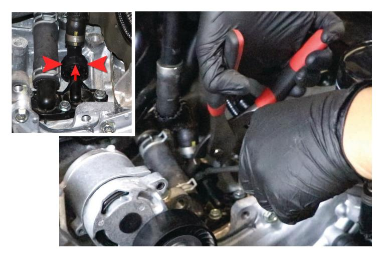
DO NOT remove the bolts on this vent. There is a single use gasket underneath.
