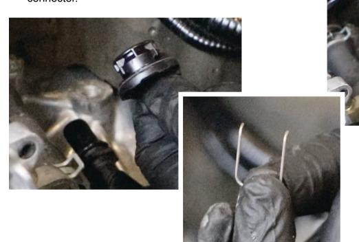
**c.** Remove air box duct using a flathead screwdriver to remove the two pins. Pull towards you to remove. This gives you better access to the front of the engine, where the other end of the PCV Hose is connected.
