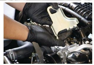
Reconnect the connector on top of the AC
