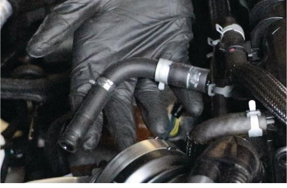
15. Slip over a supplied worm clamp on to the end of the 24" 3/8 PCV Hose, then push the hose on to the open port on top of the block. A thin layer of grease/lube rubbed inside the hose will help make this easier. Tighten clamp with a flathead screwdriver or 7mm socket and ratchet.
