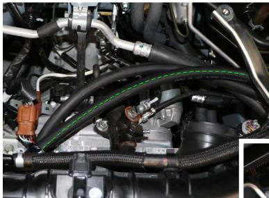
Connect the other end of the hose to Port #3 on the AOS. Slip over a supplied worm clamp, push the hose on to the port, then position and tighten the worm clamp with a flathead screwdriver or 7mm ratchet and socket.
