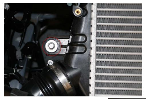
**c.** Remove mounting bolt on the driver's RH side of the intercooler using a 12mm socket and ratchet.
