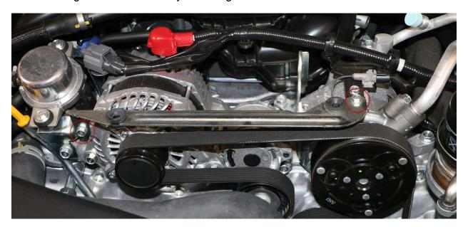
**5.** Release AC Compressor Belt by using a 14mm short socket and ratchet to turn the pulley circled clockwise. Hold the pulley while you pull the belt off of the AC compressor pulley.
