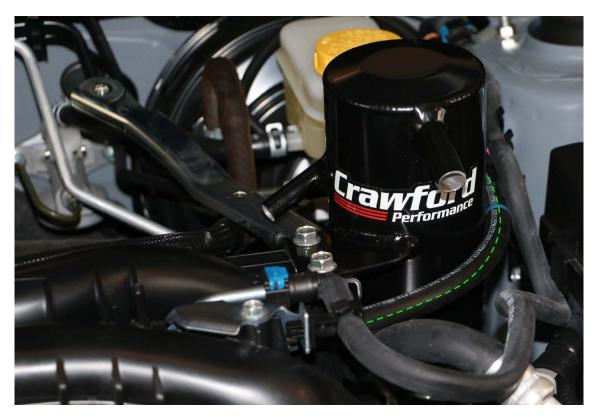
**c.** If the fuel line marked in green is too tight around the canister, use the longer 20" replacement hose included in the kit.
