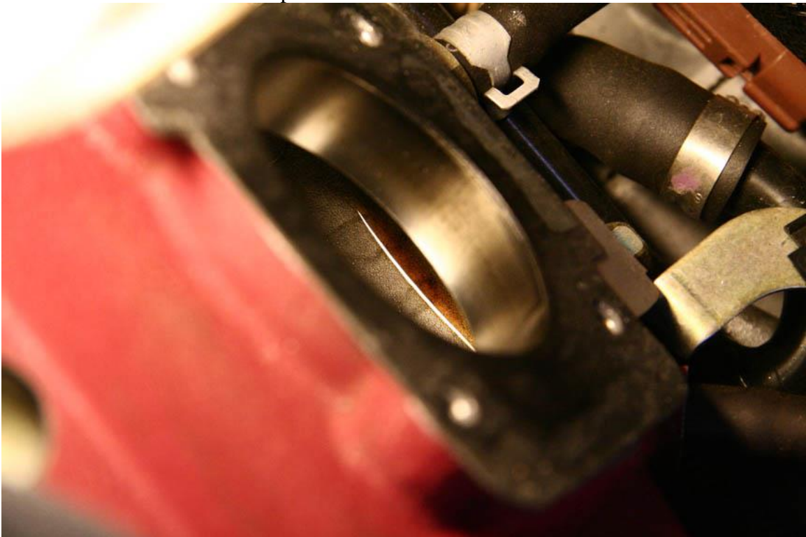
17. Notice the oil at the bottom intake manifold from the OEM engine breather system
