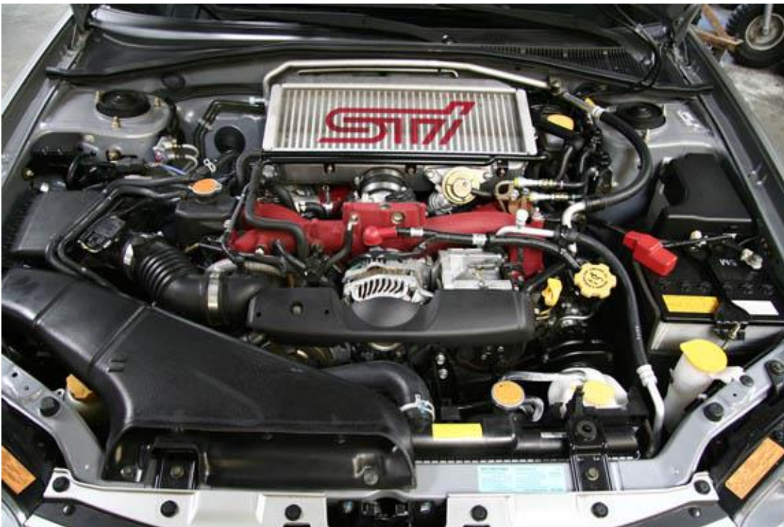
The top mount intercooler needs to be removed to easily install the Air/Oil Separator.
