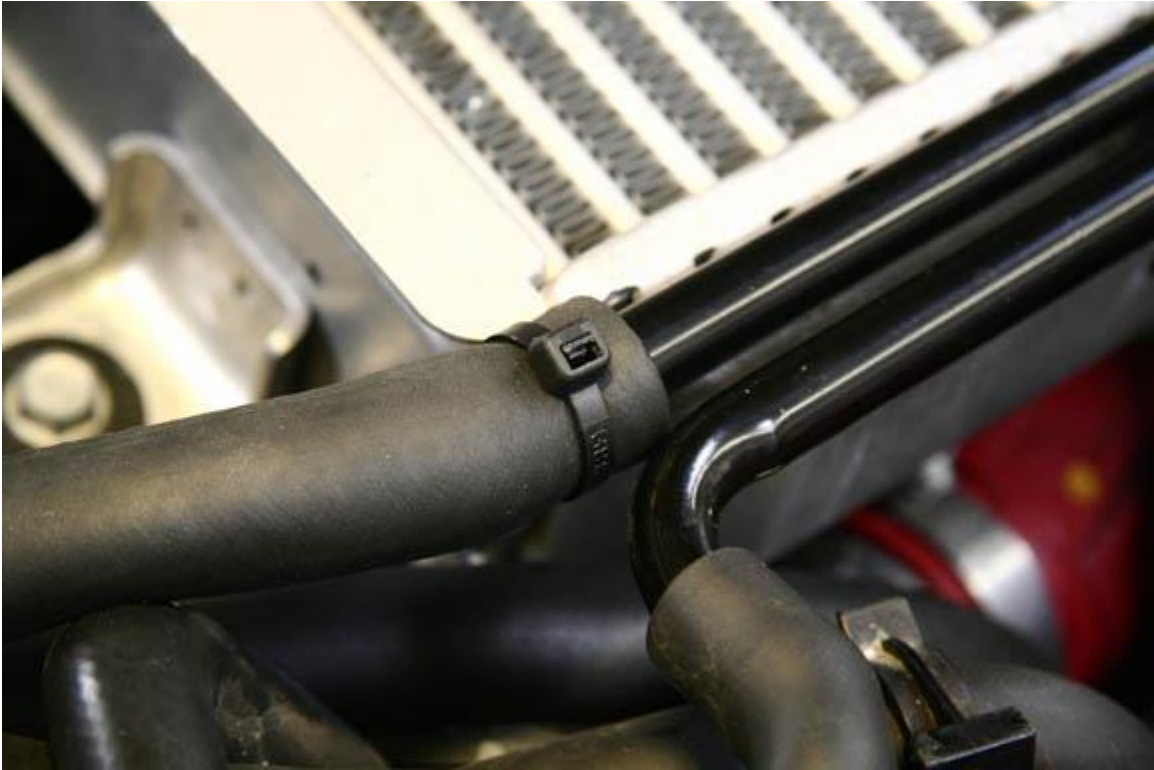
45. After connecting the hose to the cross over pipe, zip tie it to the pipe to make sure it is secure.
