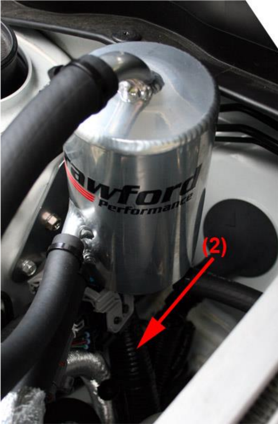
26a. There is a metal bracket that must be removed and the whole wiring unit must be rerouted along w/ the smaller wire to avoid getting in the separator's way.
