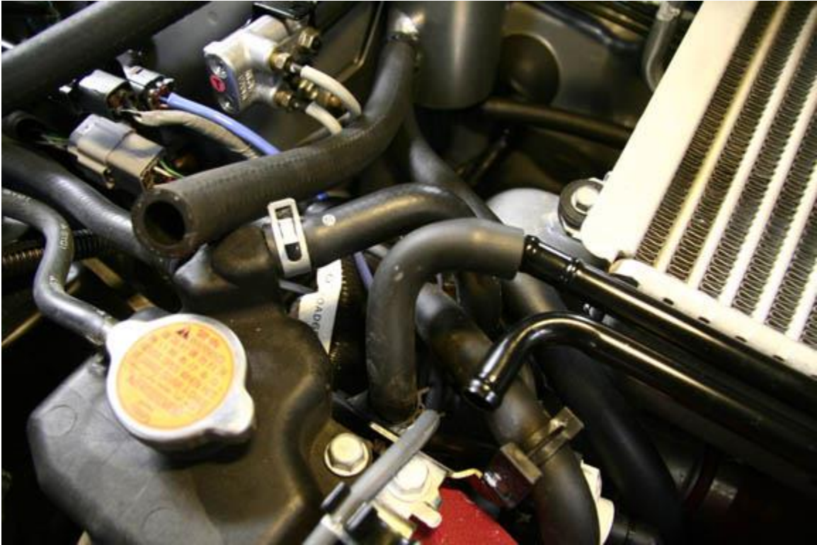
37. Screw in the right side bolt to the intercooler mounting bracket. Note the “standard” location of the OEM engine breather.
