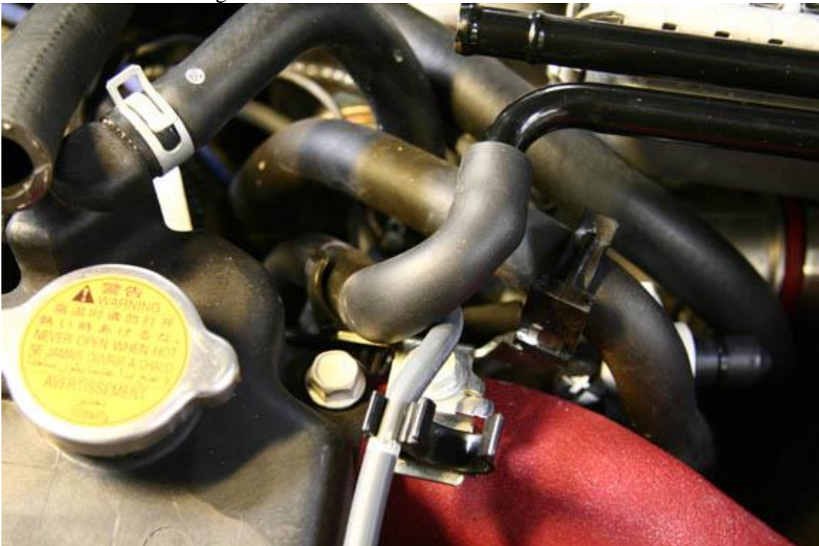
38. Place the left hand side OEM engine breather on the black cross that faces the front of the vehicle.
