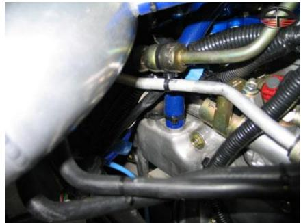
On the passenger side head, connect the hose for the air/oil separator on the front exhaust port of the head, closest to the AVCS controller.
