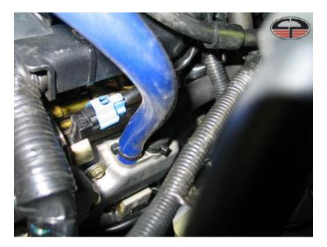
On the driver's side head, connect the hose for the air/oil separator on the front exhaust port of the head, closest to the AVCS controller. Both sides of the head will connect to the "T" and that connects to the top inlet hole on the Air/Oil Separator.
