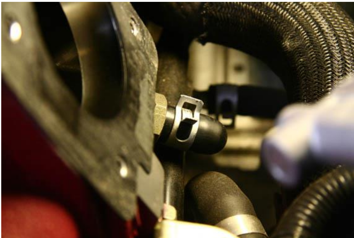
19. Remove the PCV valve and replace with 1/4" pipe plug.
