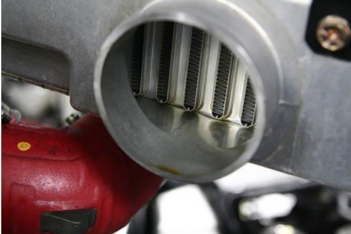
* Note the oil in the intercooler from the OEM engine breather system
