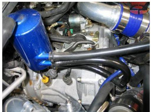
Above is the basic layout of the hoses and connectors. Note the "Y" connects to the crank case breather. The large 3/4" hose connects to the top of the Crawford Air/Oil Separator and routes over the to intake pipe.
