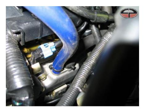
On the driver's side head, connect the hose for the air/oil separator on the front exhaust port of the head, closest to the AVCS controller. Both sides of the head will connect to the "T" and that connects to the top inlet hole on the Air/Oil Separator.
