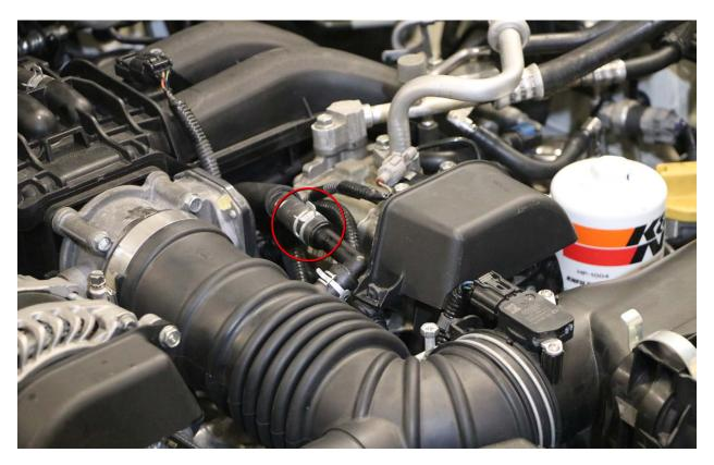
**b**. Pull smaller tube out of the larger intake tube.
