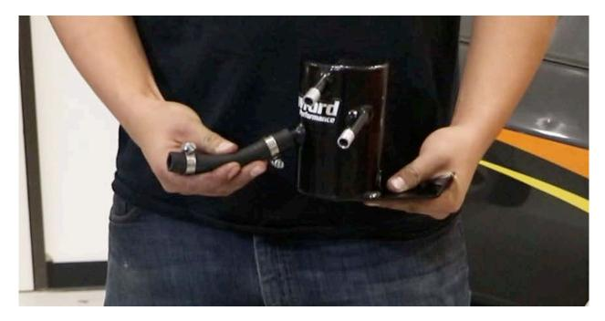
**b.** Attach the other end of the 5" Hose to the open port on top of the intake manifold\*, so that the AOS canister bracket bolt holes line up and rest where the bolts were removed on the strut braces.
