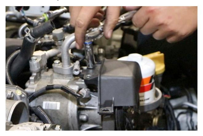
**b.** Unclip connector by pushing on the top tab to release. Disconnect connector from cover by twisting it out. Set cover aside.
