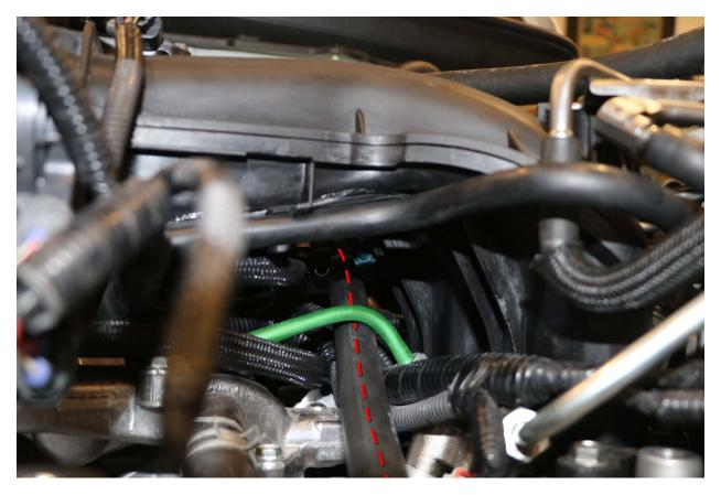
See where hose comes out on the back side (towards firewall) of the intake manifold.
