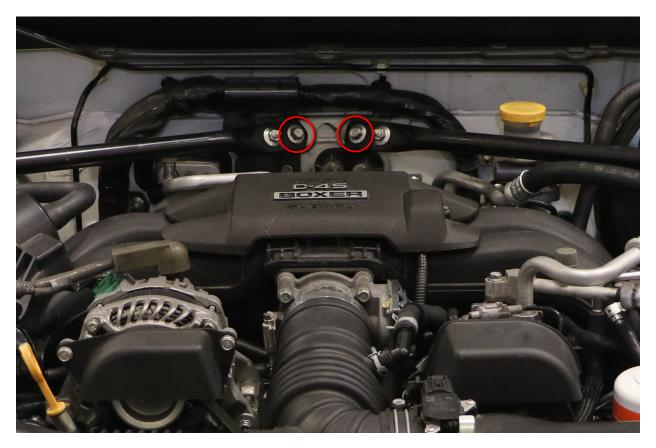
**4.** Disconnect driver's right hand PCV hose from the top of the intake manifold. Picture below is from the POV of facing the engine bay.
