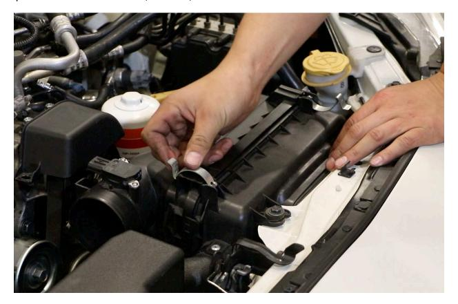
10. Disconnect AC Compressor cover at the points shown below.
