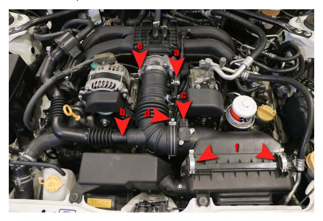
**a.** Using pliers, open the clamp on the intake hose before the throttle body, and slide it away from the end of the hose. Pull hose off, leaving clamp on the hose.
