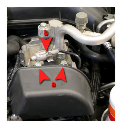
**a.** Remove 2 bolts using a 10mm socket and ratchet.
