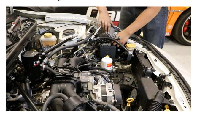
12. Remove the other end of the intake hose, by opening and sliding the clamp with pliers.
