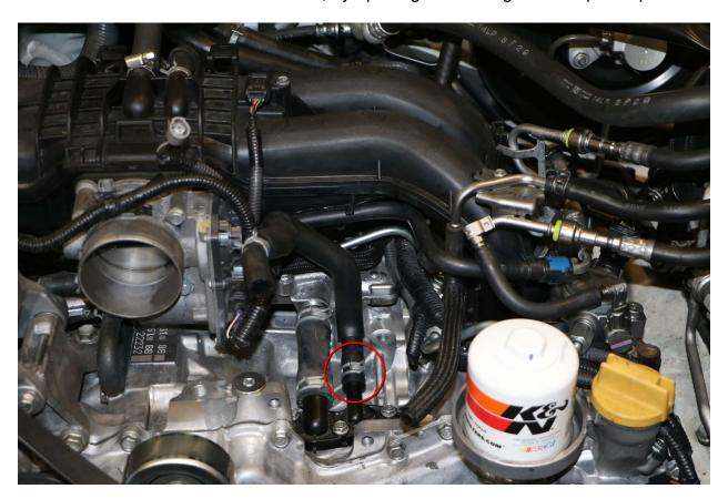
Pull off hose. This component will not be reinstalled, but we recommend storing it in case you need to later revert your vehicle back to stock.
