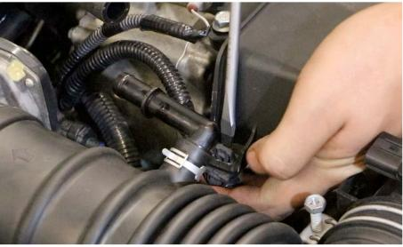
d. Loosen stud with a 10mm socket and ratchet, or a phillips screwdriver.
