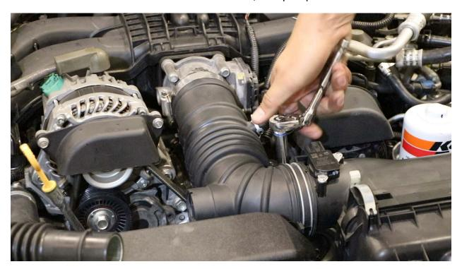
**e.** Loosen clamp using a flathead screwdriver. You can now remove the intake assembly by pulling it off the throttle body, then pulling it off the air box. Set aside.
