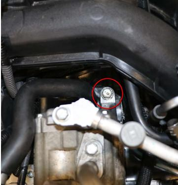
c. Lift AC compressor up and rotate it clockwise to rest on the driver's left hand side of the engine bay. Be sure not to keep the compressor in this position for a prolonged period of time to avoid kinking the hoses attached.
