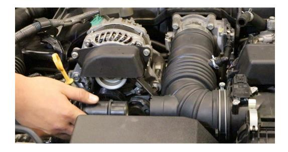
**c.** Detach MAF Sensor plug by pushing down the top tab, then push the plastic cap out of the 2 tabs: one behind the sensor and the other on the AC Compressor Cover.
