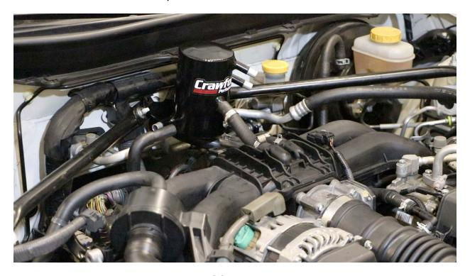
**6.** Replace the 2 strut brace bolts with the AOS bracket lined up with the bolt holes. Tighten to OEM torque spec, using a 12mm socket and ratchet.
