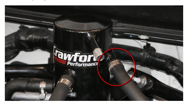
**15.** Slip a supplied worm clamp over the other end of the hose on top of the crankcase. Push hose on to plastic port\*, slide clamp in to place, and tighten using a flathead screwdriver so that you cannot pull the hose off by hand.
