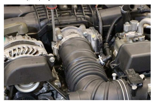
f. Unclip both sides of the air box, remove, and set aside.
