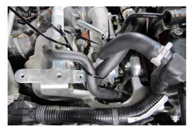
In order to make it easier to access these bolts, use zip ties (or other methods) to pull the hoses out of the way.
