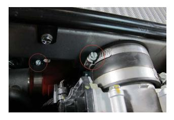
**c.** loosen screws on the rear clamp on throttle body hose, and on the turbo inlet clamp underneath
