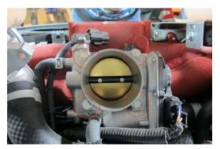
**b.** Remove four 10mm bolts from the back of the throttle body housing
