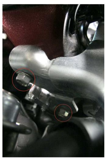
Pictured are the 2 bolts that are used for mounting the canister.
