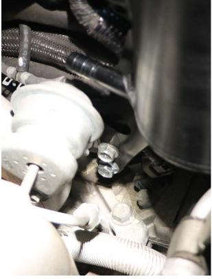
**11.** Behind the Intake Manifold on top of the block, locate and disconnect the 2 plugs circled below. Push down tabs and pull apart.
