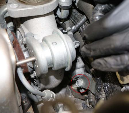
Then, remove Bolt with a 12mm Ratcheting Wrench. You can use the Socket/Ratchet, but it may bind against the oil line.
