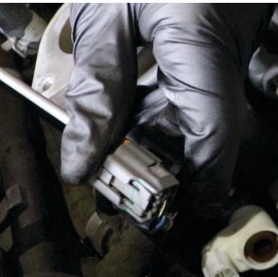
**15.** Remove the black side of the connector from the hose by releasing the locking clamp on the hose with a flathead screwdriver, and pulling out the connector.
