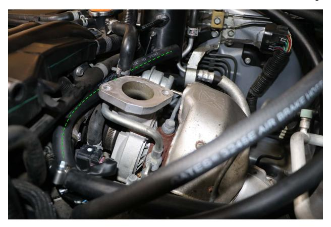
**23.** Slip over a supplied clamp onto the end of the 13" 1/2" Vent Hose, and push hose onto Port #4 on the AOS. Slide clamp to end of hose, and tighten using a flathead screwdriver. Check that the hose cannot be pulled off the port by hand.
