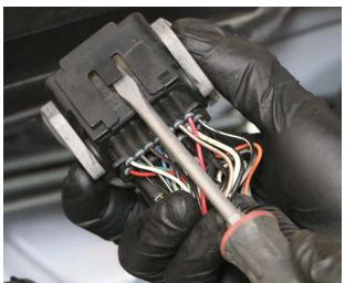
**a.** Release Main Harness Connector from Bracket by pulling down on tab underneath, and sliding connector off of its mount.
