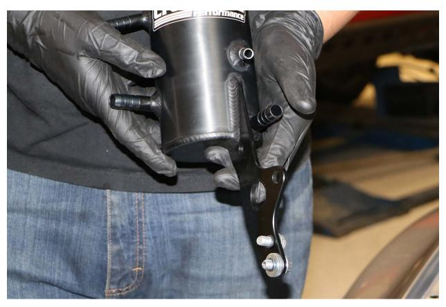
Place the 3 supplied washers on the bottom bolt, then secure both bolts with the supplied o-rings to keep them in place while mounting the canister.
