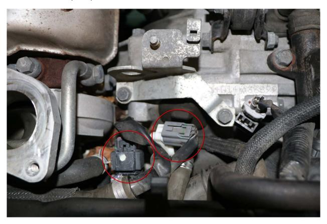
**12.** Locate the PCV Hose Port on top of the block beneath the plugs. Use pliers to open the clamp and pull away from the port. Pull hose off port.
