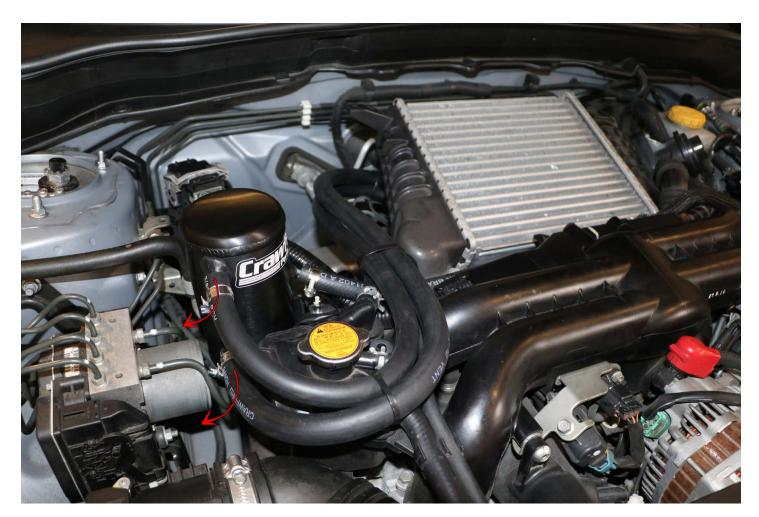
**37.** Start your car and check for any leaks. Your car may change RPM's to adjust to the new setup, but should level out and run smoothly soon after. If you have a rough idle, it is possible you have a vacuum leak.
