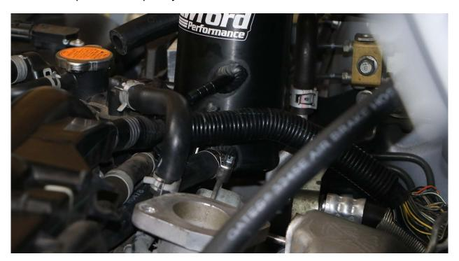
**24.** Route 20" 3/8" PCV Hose underneath the 2 longer hoses, and then along the same path as the 13" hose just attached, under the coolant line but above the wire harness.
