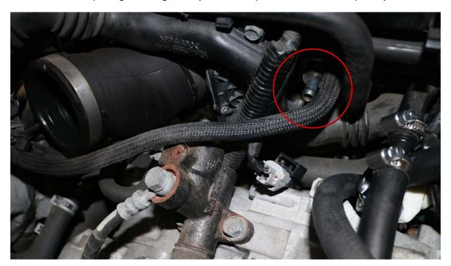
22. Route 13" 1/2" Vent Hose in front of turbo / under coolant line as shown below marked in green.
