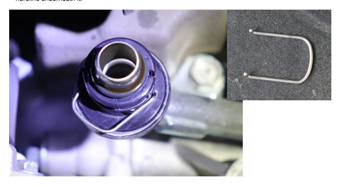
5. Cut the same 5/8" line just in front of the bulge point shown below. Remove this line once cut.
