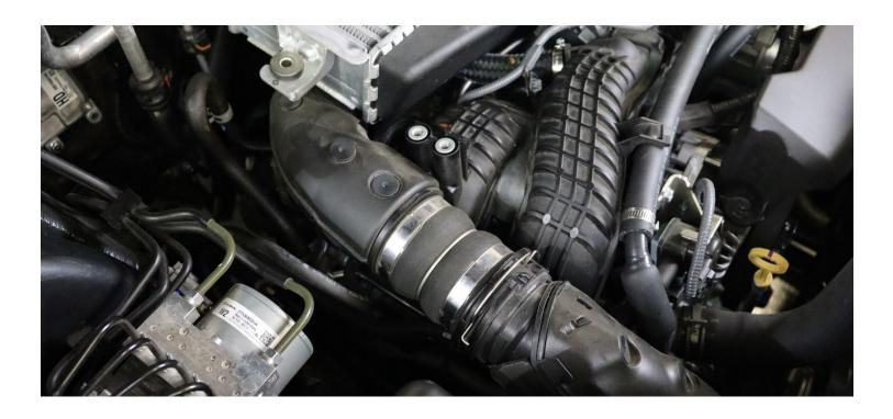
17. Line up the intercooler mount brackets and reinstall the original 12 MM bolts removed in step 1 to fasten the intercooler in place.
