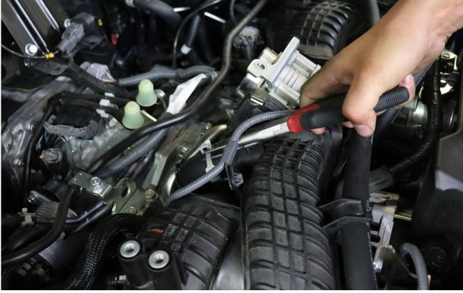
12. Next remove the metal clamp on the lower port of this line with a set of pliers. Once loose, pull the PCV hose out of the vehicle. Both ports should be exposed and ready to reciev the AOS hoses.
