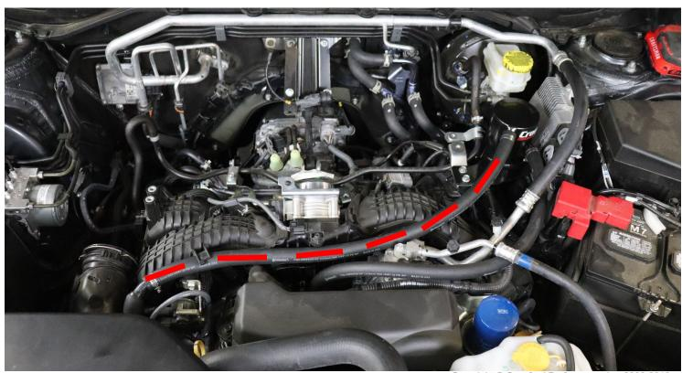
11. Moving to the backside of the intake manifold, you will need to remove the PCV hose connected to the manifold as shown. Squeeze the metal clip with a set of pliers to remove the hose.
