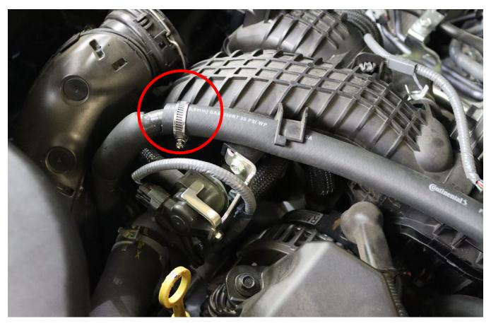
10. Fasten the 5/8" hose from step 9 to the top port on the AOS cannister. Once fastened, Route the line across the intake manifold as shown.
