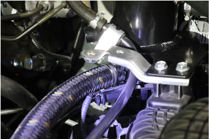
15. Next route the 29" length of 7/8" hose from the manifold to the upper 7/8" port on the AOS cannister.
