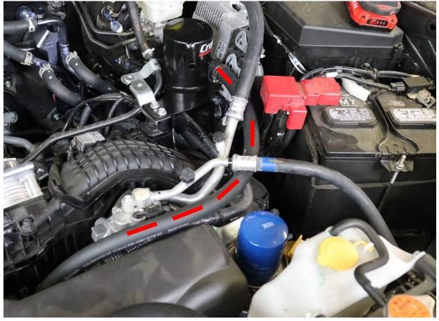
8. Fit the 1/2" Hose over the port revealed in step 4 and sinch down with one of the provided hose clamps. Repeat for the cannister port
