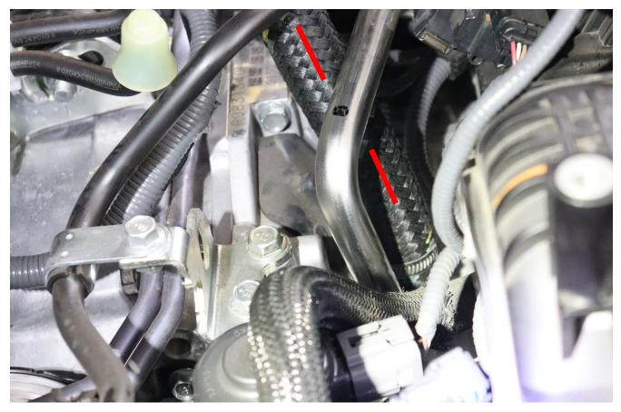
14. Route the 21" length of 7/8" hose from the block to the lower 7/8" cannister port and fasten with hose clamps.
