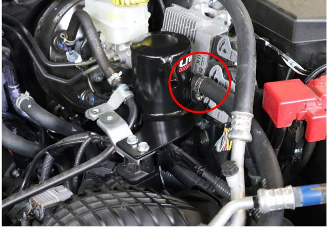
9. Fit the provided 29" length of 5/8" ID tube to the hose that was cut in step 5. Fasten with a provided hose clamp.
