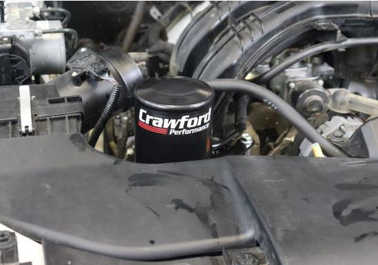
9. Route the 20" hose on the top of the cannister under the manifold as shown. This line will connect to the intake manifold, while the 12" hose will connect to the PCV port on the block.
