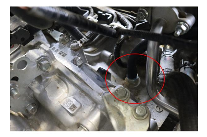
11. Route the 20" hose to the intake manifold port shown in step 2a.
