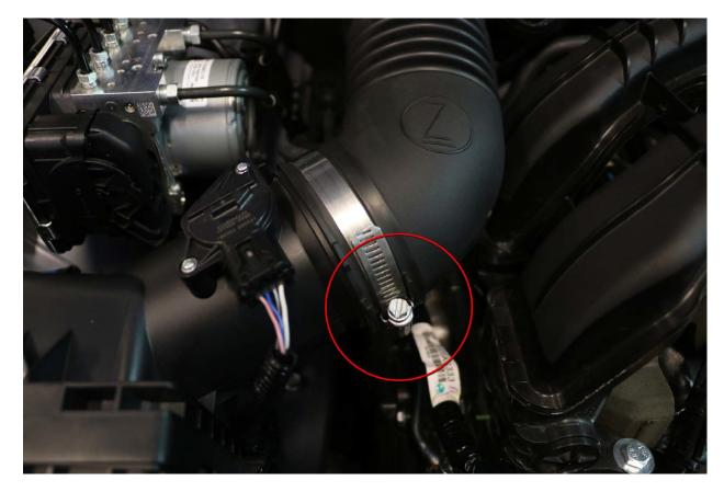
b. Use a flathead screwdriver to loosen the clamp by the throttle body
