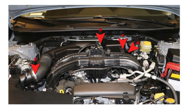
a. Use a flathead screwdriver to loosen the clamp by the air box.
