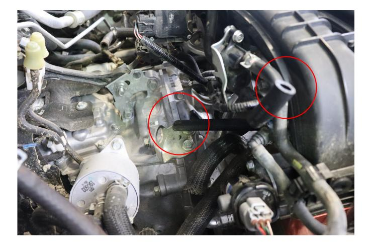
10. Route the 12" line underneath the EGR tube and to the PCV port on the engine block.
