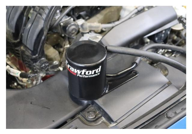
5. Fit the cannister + bracket so the bracket mounting holes are over the two intake manifold bolts that were removed in step 3. Route the 12" hose on the bottom port under the intake manifold as shown and towards the PCV port on the engine block shown in step 2b.
