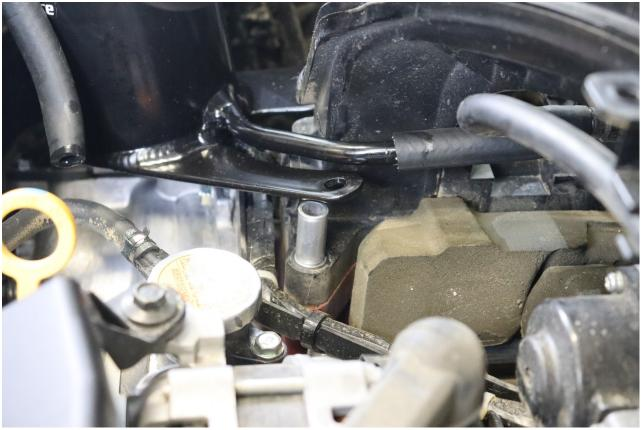
7. Tighten the provided 110 mm bolt with your fingers until it is snug against the bracket and washer. Repeat for the middle intake manifold bolt that was also removed. Remember this middle bolt does not require a spacer if the BPBs are installed.
