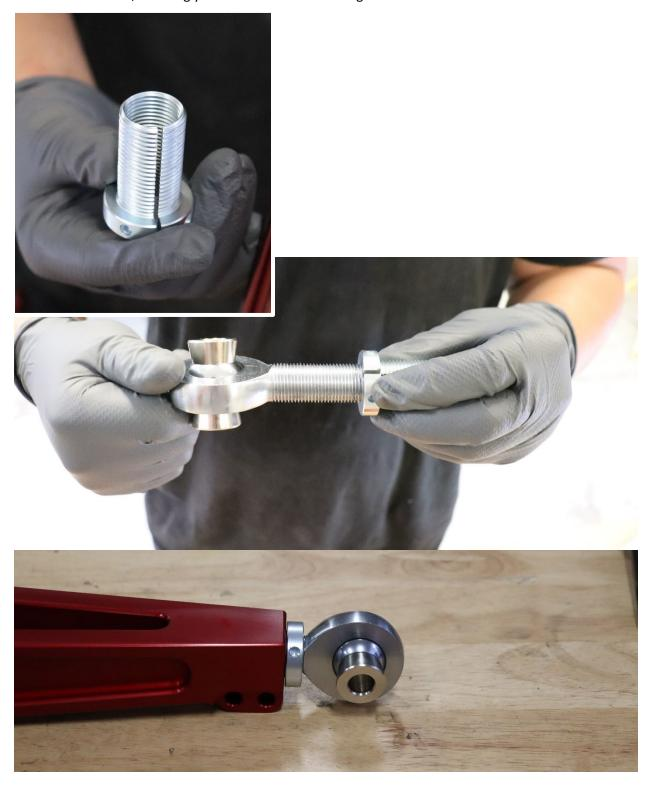
8. Install 2 of the provided 8 mm 12-point bolts into the locking joints on the control arm and fasten with the provided 10 mm 12-point nuts.
