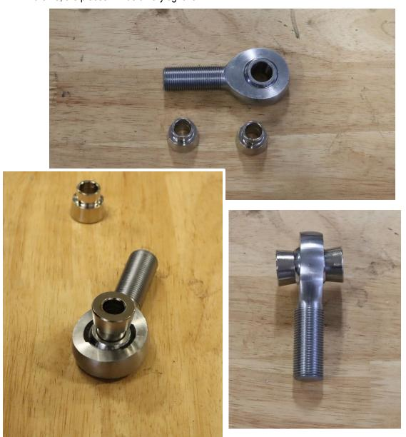
7. Apply anti-seize to the heim joint threads and install the heim joint into the alignment sleeve completely, so that the heim joint has no threads showing. Then apply anti-seize to the adjustment sleeve and proceed to thread the interlocked heim joint and alignment sleeve into the control arm. When threading the alignment sleeve, heim joint combo, the threading will be left-handed, meaning you need to turn it left to tighten it into the arm.
