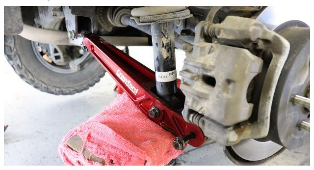
13. Tighten the three lower control arm bolts to 90 ft-lbs. Finish by fully lock the heim joint into position. To do so, tighten each bolt to 30 ft-lbs. 3 times in sequence, outer then inner bolt 3 times. (17 mm socket, Torque wrench, 17 mm standard wrench, 8 mm ratchet wrench, 10 mm socket)
