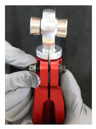
9. Install the heim joint to the chassis using the OEM 17 mm bolt removed in step 4. Do not tighten yet. (17 mm ratchet wrench, 17 mm standard wrench) Be consistent with the direction your bolts face, either towards the front or rear of the car.
