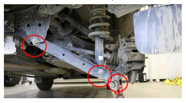
4. Undo the 3 lower control arm bolts and remove the arm. A jack stand may be needed to relieve pressure off these bolts to make their removal easier. If you use power tools, be sure not to strip any hardware. Repeat for the driver side. (17mm ratchet wrench, 17 mm standard wrench)
