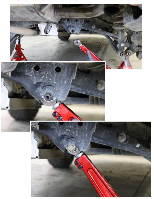
10. Using a provided 17 mm bolt, swing the control arm into position and install it onto the rear shock as shown.
