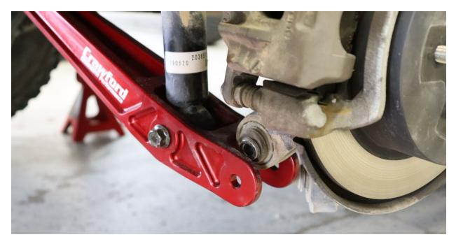
12. Using the floor jack and a support of some kind (we used a wood block covered with a rag) you can align the hub to fit into the control arm. This will take some finesse and patience due to the tight fit. Use a long screwdriver if necessary, to align the hub joint so that it will slide between the control arm mounts when lifting up on the shock with the floor jack. The hub should slide into position, allowing the bolt to be inserted.
