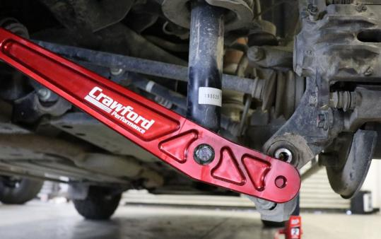
11. Aligning the rear hub into the control arm will require a floor jack to compress the rear shock and bring the control arm into position so that you can insert the provided 17 mm bolt and secure the hub to the arm.
