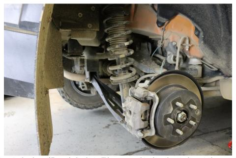
3. Locate the three 17 mm bolts that will be removed to drop the stock control arm out of the vehicle.
