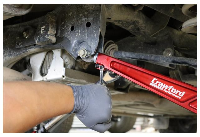
14. Double check all hardware to ensure nothing is left loose. Repeat this process for the other side of the vehicle. We Recommend keeping any OEM parts removed just in case this install needs to be undone.
