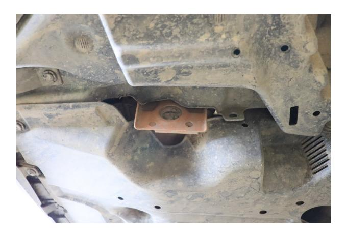
3. Clear debris and dirt out of the mounting points.
