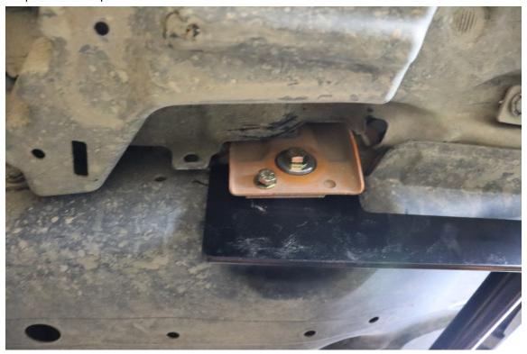
9. Place a 3/8" washer over the exposed 3/8" bolt end.
