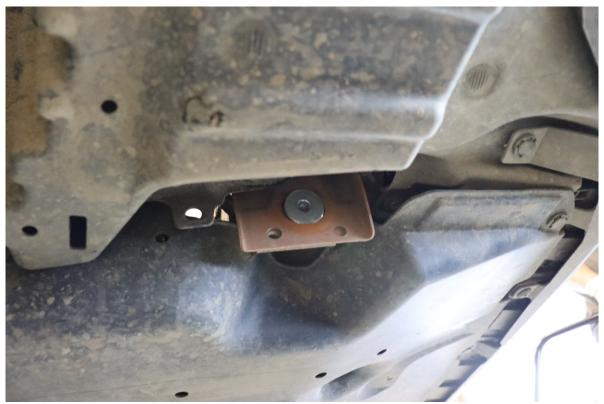
5. Steps 5-10 will be easier with a friend to help support the bumper in place. **Note:** Only the passenger side of the vehicle is shown, but the process in steps 5-10 is the same for both sides. Lift the bumper so the mounting tabs are positioned on the inside of the vehicles mounting points. Place a 5/16" washer over the provided 5/16" bolts and push it through the step-down spacer and
