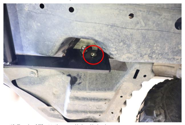
10. Thread on 3/8" nut to the exposed bolt end by hand.
