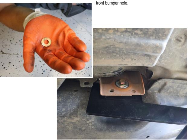
6. Place a 5/16" washer on the exposed 5/16" bolt on the inside of the bumper.
