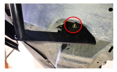
7. Thread on the 5/16" nut to the exposed bolt end by hand.
