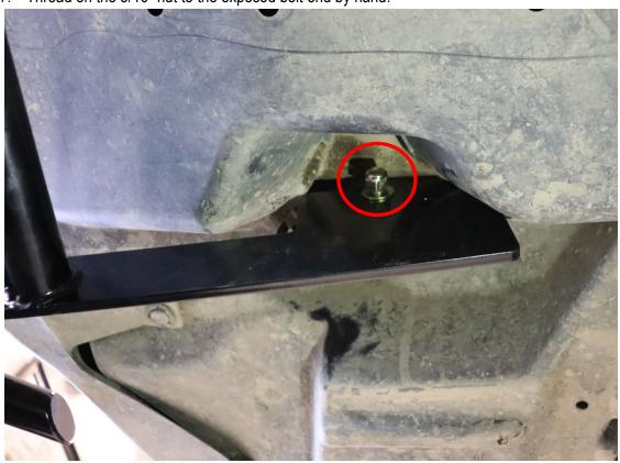
8. Place a 3/8" washer over the provided 3/8" bolt and push it through the rear hole on the mounting plate and bumper.
