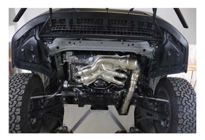
6. Locate the mounting positions for the skid plate and mount the plate using the provided 50 MM flange bolts . If you are using jack stands, use a floor jack to lift the skid plate into place and thread the provided flange bolts by hand. If you are on a lift, put the plate into position and thread in the bolts by hand.
