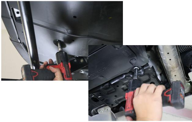
5. If the Crawford Performance front bumper is installed, leave it hanging and work the OEM skid plate out from underneath the bumper. If you do not have our bumper, then simply drop the skid plate out of the vehicle.
