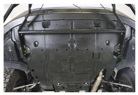
2. If you have the Crawford Front Bumper installed, follow these steps to move it out of the way of the OEM Skid plate. First remove the larger ½" mounting bolts shown below. Once removed, the bumper will naturally want to swing down. Disconnect the lights (if installed) and let the bumper hang. (1/2" Socket + Wrench)
