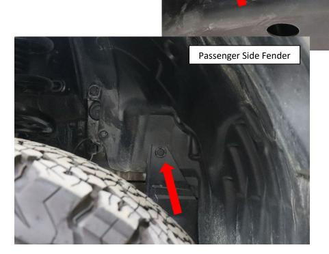
4. Remove the four 12 MM Bolts holding the skid plate to the sub-frame. (12 MM Socket)
