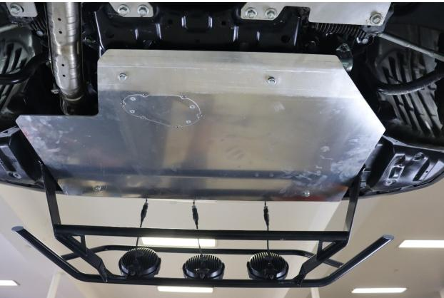
7. Torque down the flange bolts to 25 ft-lbs. (12 MM Socket)
