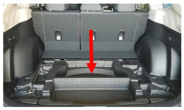
**22.** Locate the plastic push clips holding the foam tool holders in place. Remove these clips and set the foam pieces aside.
