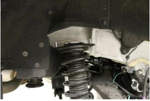
**28.** Locate the Crawford Performance strut extension. Install the short stud extensions provided to top of strut and torque to 30 ft-lbs. (16mm box wrench). Add thread lock before installing stud extender
