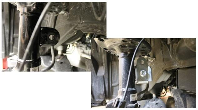
**16.** Install the 1/4" thick spacer washer onto the end link.
