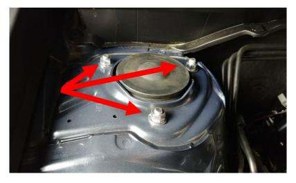
8. Remove factory strut assembly from vehicle
