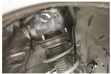
9. Locate the Crawford Performance front strut extension. These are universal and fit the passenger and driver side equally. Apply a drop of Loctite to the strut studs and thread on the strut stud extensions (16mm box wrench). Torque to 30 ft-lbs. and slide the spacer onto the top of the strut.
