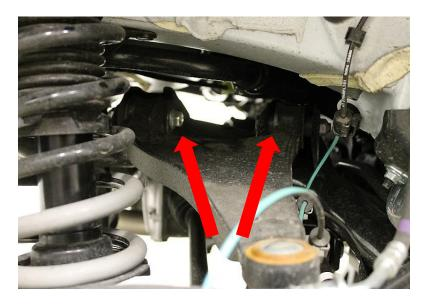
25. Loosen but do not remove the front lower control arm bolts (17mm socket)
