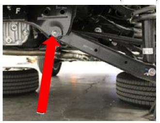
27. Remove both the factory lower rearward control arm bolt at the knuckle and the factory lower strut bolt (17mm socket), then lower the control arm and remove the factory strut assembly from the vehicle Warning: Hold strut assembly while lowering the control arm
