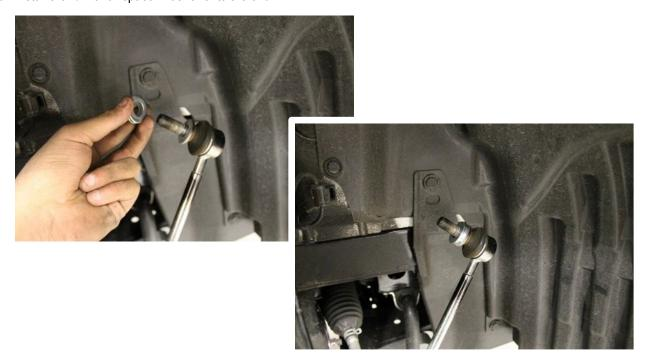
**17.** Install the factory end link to the Crawford Performance bracket using the factory hardware (18mm socket). Torque the bracket and end link to 45 ft- lbs.
