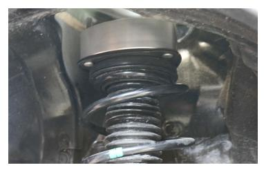
11. Align the three upper strut stud extension threads into the holes on the vehicle and fasten utilizing the provided M10 x 1.25 strut flange nuts. (14mm socket) When installed correctly, the Crawford Performance logo will be legible through the strut tower when facing the engine compartment. (Driver side shown)
