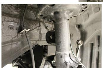
3. Remove the brake line bracket at the strut body (12mm socket). Let hang out of the way. Note how the brake line is run from the underside of the strut body. Installation will be changed in a later step.
