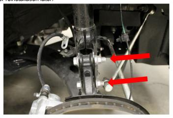
**6.** While keeping the lower control arm supported, release the knuckle from the strut body and let hang out of the way. Make sure to not overextend the ABS, brake line, and CV axle. Adjust as necessary.
