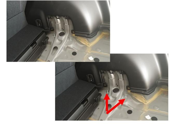
**24.** Loosen but do not remove the upper control arm bolts (17mm socket).
