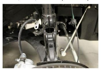
7. Remove the upper strut hardware (14mm socket). Make sure to hold the strut assembly from falling out of the vehicle. A helper is recommended for removal.
