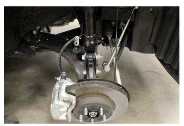
13. The cam bolt has lines that correspond to a notch on the strut body (paint marked for picture clarification). You will rotate the cam bolt until the lines are facing the inside of the vehicle. Line up the last line with the notch. This sets max negative camber. Torque both bolts to 95 ft-lbs (19mm socket + 19mm ratchet wrench). Final adjustment and torque to be set by the alignment tech.
