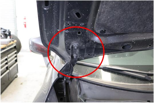
2. Remove lower hood bracket nut on one side of the vehicle (12 MM socket, 3/8" nut driver). **Perform this on one side at a time to avoid misaligning the hood.**
