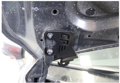
4. Make sure bracket is tightly fastened to the hood. Repeat for the opposite side of the vehicle, making sure to only remove specified fastening hardware.
