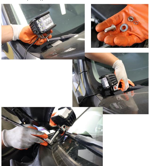
2. Once the pod is mounted, route the wires so that they fit snugly against the hood bracket as shown. Use a zip tie to secure the wires into this position. Placing them here will allow for slack and enough space to open the hood without tugging at the wires. Fasten the hood pod wire to the zip tie on the pod bracket mentioned in part one of this install. Repeat step 1 and two for the driver side
