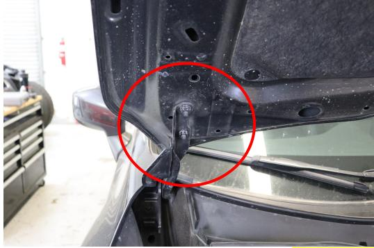
2. Remove lower hood bracket nut on one side of the vehicle. (12 MM socket) **Perform this on one side** at a time to avoid misaligning the hood.
