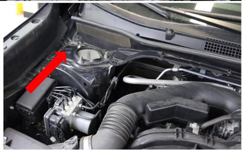
11. Next will be routing the on/off switch to the interior of the vehicle. Start by removing the plug in your firewall behind the master brake cylinder. The hole is shown below after the plug is removed.
