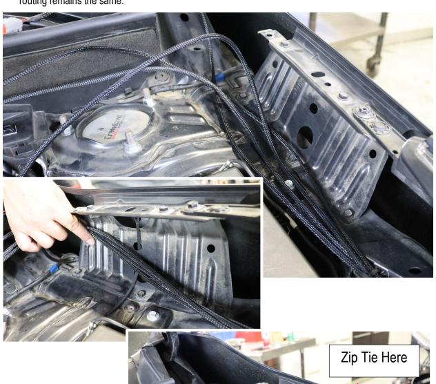
10. Clean off the areas indicated below in preparation for sticky tabs to be placed. Once cleaned, place down the tabs. **Do not** fasten any wires into them yet.
