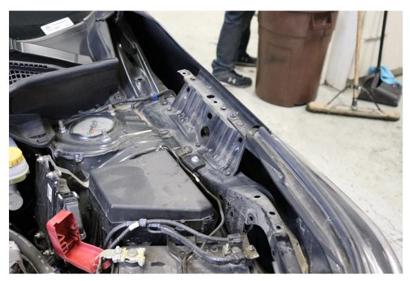
9. Route your plug and switch wires towards the top of the engine bay as shown. Loosely zip tie the bundle to the fender support indicated below, allowing enough slack for the switch wire and passenger hood pod wire to be installed. Leave the short pod connection wire near the driver side hood bracket. You should only have 3 wires with this kit, we have an extra shown for another component, but the routing remains the same.
