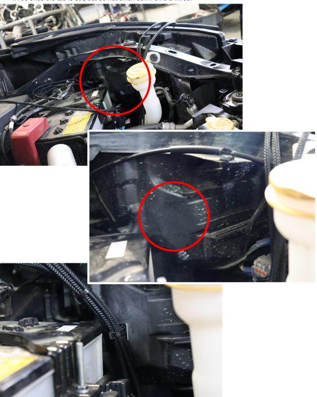
8. Remove the plastic fender trim on the driver's side of the engine bay by releasing the indicated plastic clips. (Flat Head Screwdriver)
