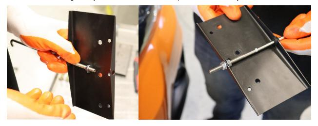
4. Attach the hood light pod relay to the relay plate. (position on the plate does not matter)
