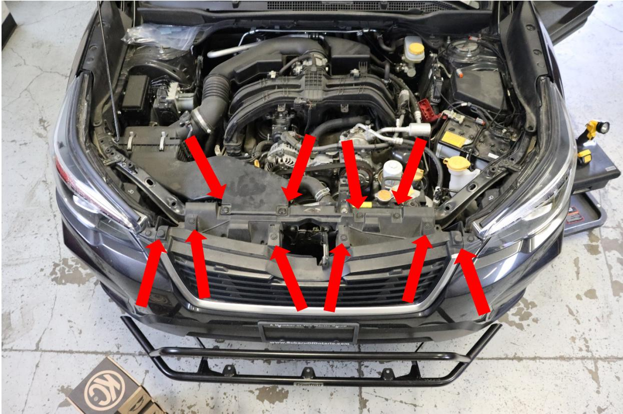
18. Remove the air filter inlet tube.
