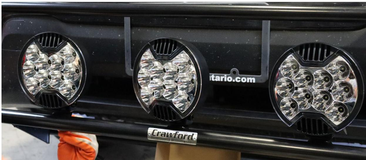
26. Clean the lower bumper lip in preparation to receive sticky tabs to mount the light pod wires and the plugs. Mount them as they fit best for you and your vehicle. Connect lights when done.
