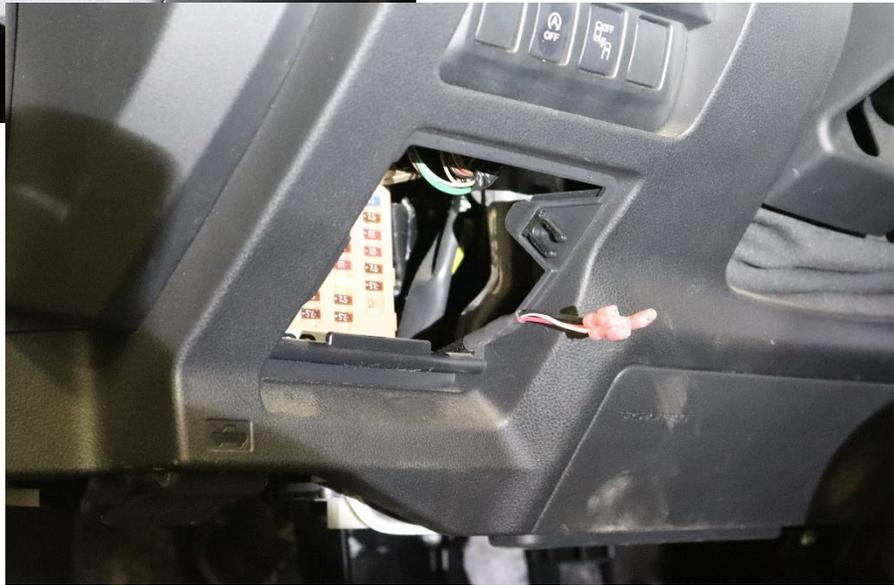
14. Drill out your fuse panel cover to receive the switch. You will need about a 3/4" hole for a tight fit.
