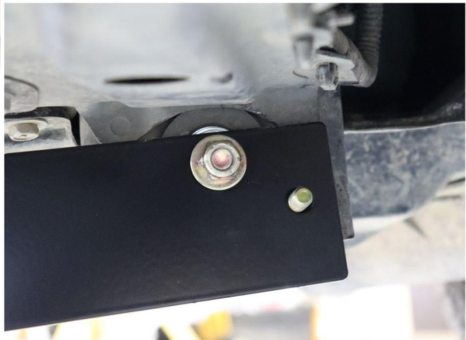
8. Place a 5/16" washer over the exposed 5/16" bolt end.
