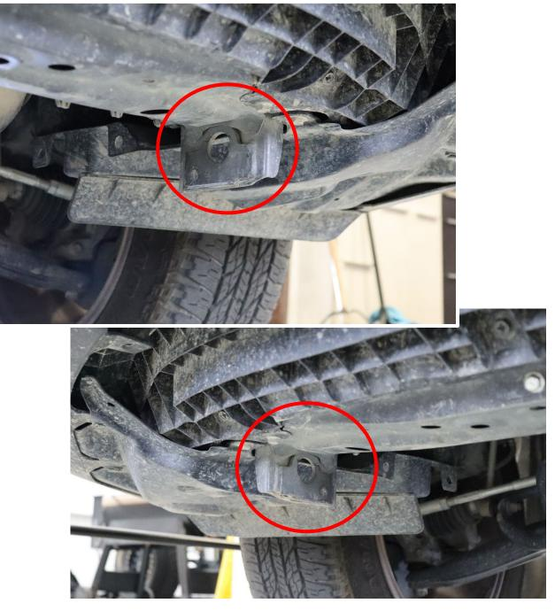
3. Insert the provided step-down spacers into the mounting points so they sit flush with the plate
