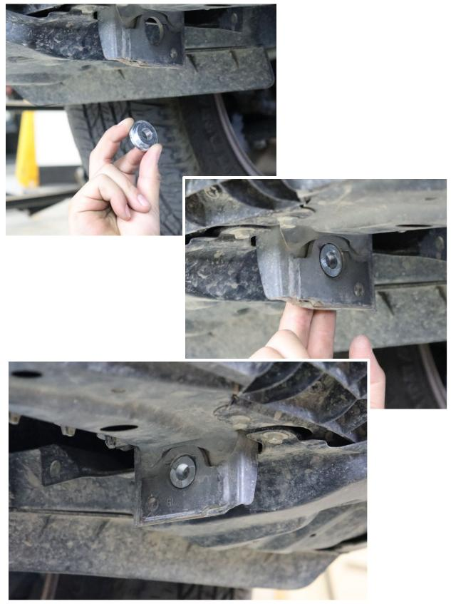
4. Steps 4-10 will be easier with a friend to help support the bumper in place. Note: Only the passenger side of the vehicle is shown, but the process in steps 4-10 is the same for both sides. Lift the bumper so the mounting tabs are positioned on the inside of the vehicles mounting points. Place a 1/2" washer over the provided 1/2" bolts and push it through the step-down spacer and front bumper hole.
