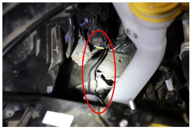
22. Fish the wire to the front grill support through the gap filled by the foam padding shown below.
