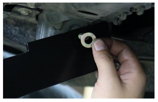
6. Thread on the 3/4" nut to the exposed bolt end by hand
