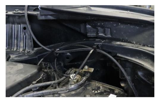
9. Zip tie the switch wire to the exposed OEM wire at the top of the fender support as shown below.
