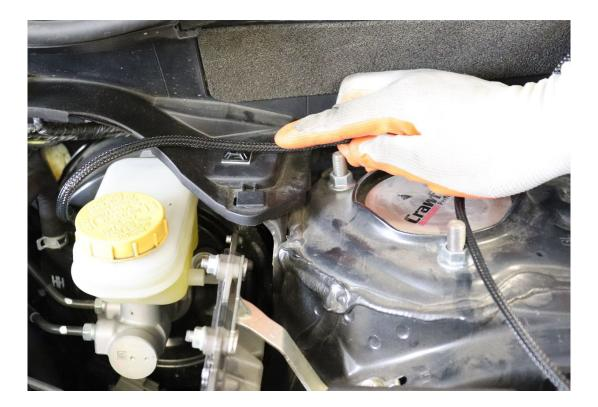
11. Next will be routing the on/off switch to the interior of the vehicle. Start by removing the plug in your firewall behind the master brake cylinder. The hole is shown below after the plug is removed.
