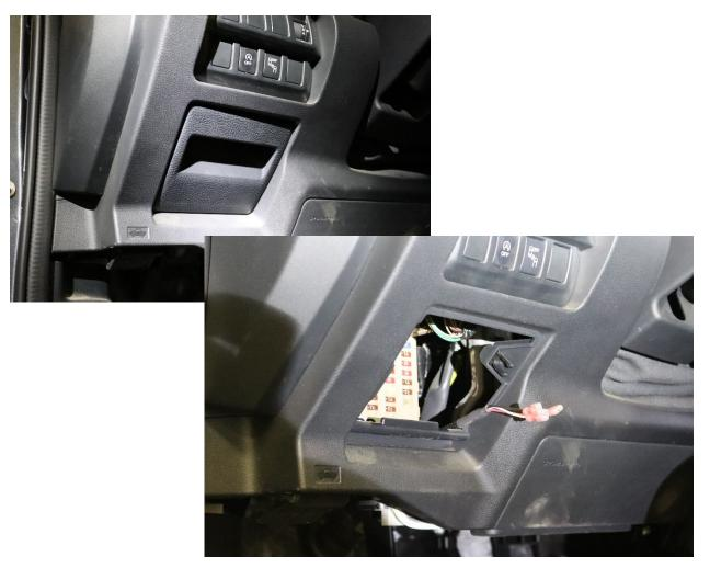
14. Drill out your fuse panel cover to receive the switch. You will need about a 3/4" hole for a tight fit.
