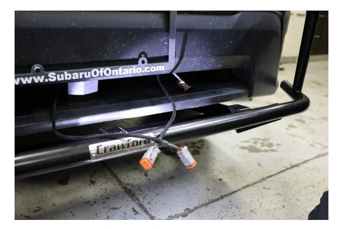
24. Once the light pod wires are located behind the bumper as shown above, the provided KC Daylighter lights can be installed.
