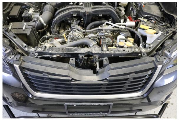
21. Next will be routing the light pod wire ends to the front of the vehicle. Start by funneling the three plugs down to the support bar behind the grill. They will be directed down to the bar through the cavity behind the driver side headlight.
