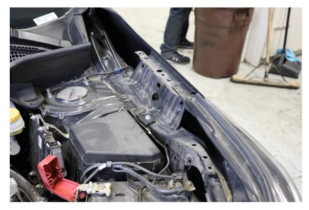
8. Prep the areas shown below to receive a sticky tab. Clean the fender support frame with brake clean or some other degreaser to get the best results. Attach tabs to the locations shown below. Fasten the wires once the tab is set, but do not cinch down on the wires. Only the switch wire and the ground wire should be routed through these tabs.
