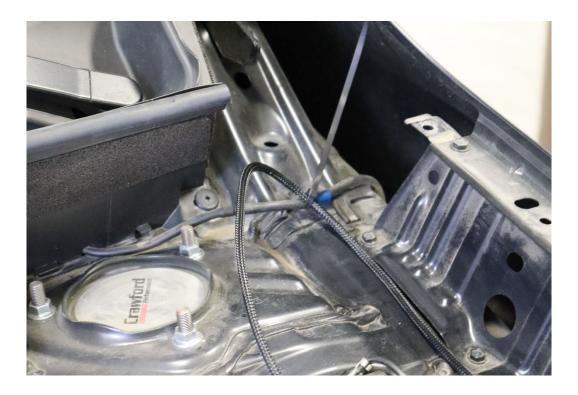
10. Clean off the area indicated below in preparation for a sticky tab to be placed down. Do not fasten any wires into the tab yet.
