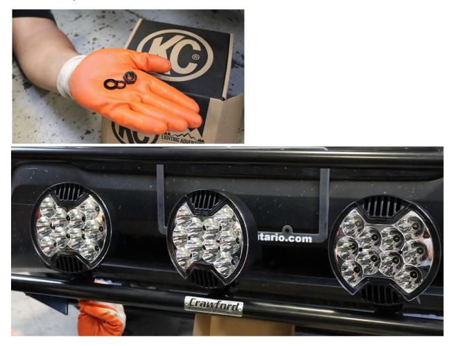
26. Clean the lower bumper lip in preparation to receive sticky tabs to mount the light pod wires and the plugs. Mount them as they fit best for you and your vehicle. Connect lights when done.
