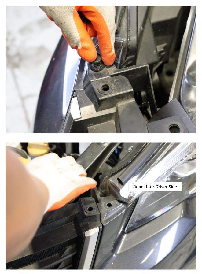
20. Once all the tabs mentioned above are removed, lift the wind deflector behind the grill and pull it out of the vehicle.
