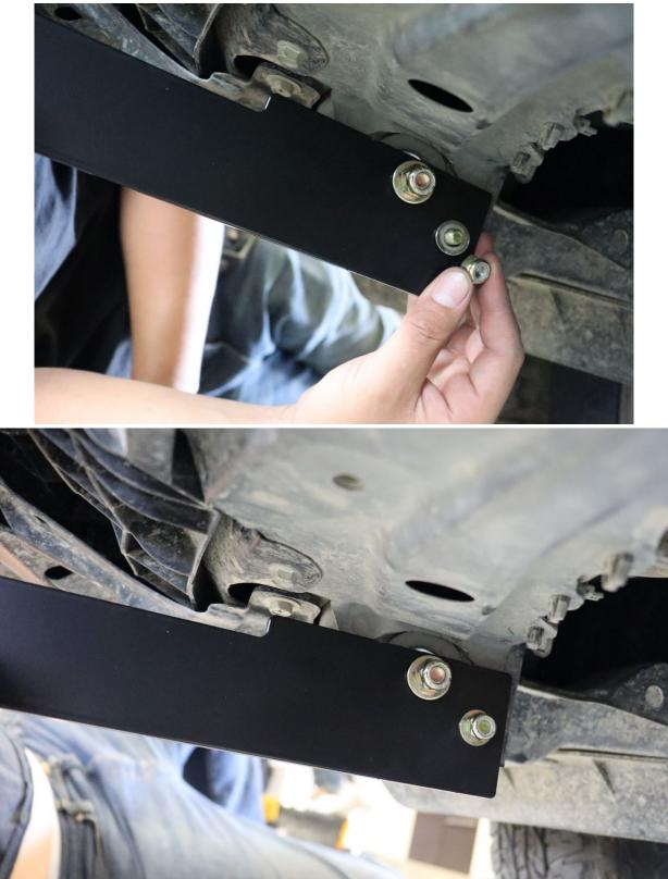
9. Thread on a provided 1/2" nut to the exposed bolt end by hand.
