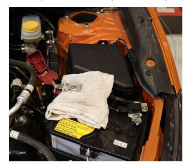
2. Remove the Battery Brace Strut. (10 MM Socket)
