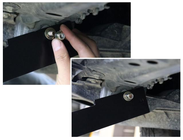
7. Place a 5/16" washer over the provided 5/16" bolt and push it through the rear hole on the mounting plate and bumper.
