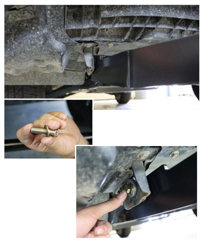
5. Place a 1/2" washer on the exposed 1/2" bolt on the inside of the bumper.
