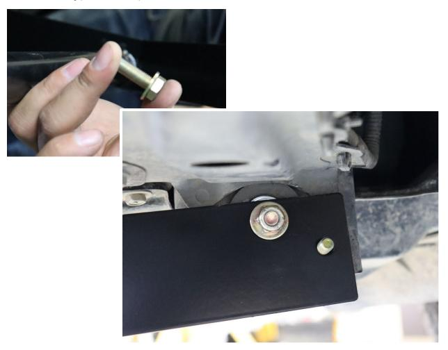
8. Place a 5/16" washer over the exposed 5/16" bolt end.
