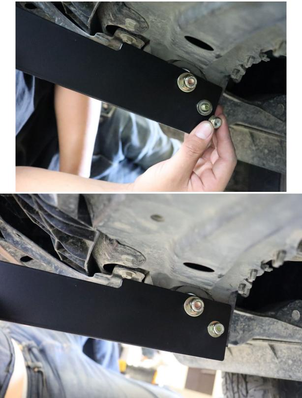
9. Thread on a provided 1/2" nut to the exposed bolt end by hand.
