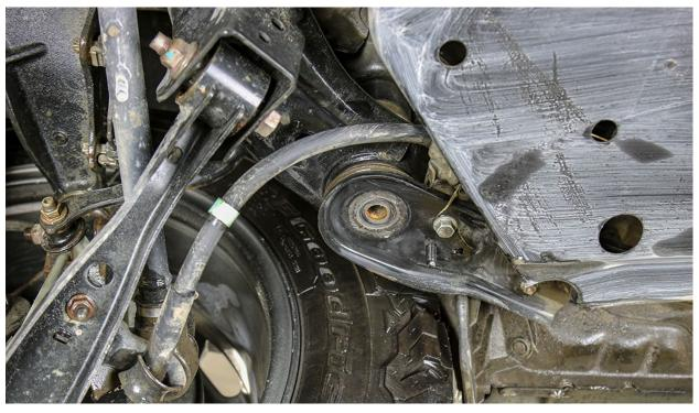
3. Locate and install the sub frame bump pads onto the rock guards. There will be 4 bump pads total, and two go on each guard. Use a 9/16" socket to tighten the pad onto the guard tabs as shown below.
