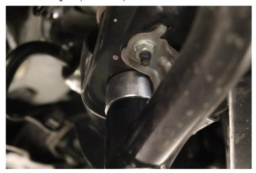
6. Tighten subframe bolts and make sure the guards are completely secure to the vehicle.
