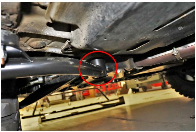
5. Install rear rock guard mount with spacer between guard mount and subframe. Use the provided 19 mm bolt to secure guard. (19 MM socket)
