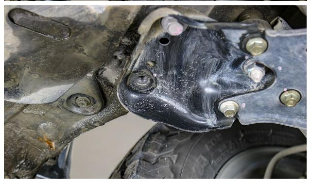
2. Remove rear subframe bolt just behind the rear tire. (19 MM socket)
