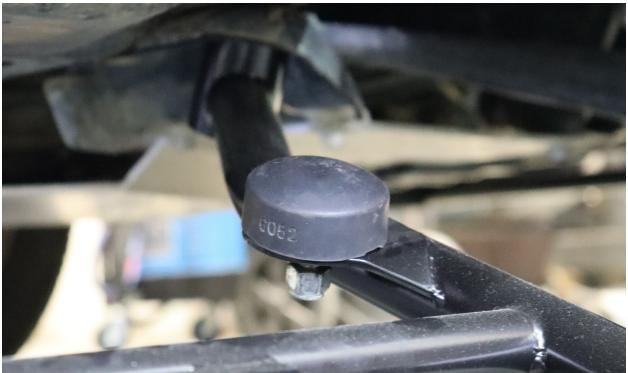
4. Install front end of rock guard mount to sub frame using OEM bolt removed in step one. (19 MM socket)
