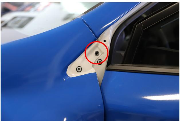
3. Pull the two mirror pod connector ends mentioned in step 20 and 25 of the harness installation through the fender well so that they are exposed in the door frame. This will make the wire connections much easier. Shown on drivers side.
