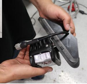
4. Slide the provided heat shield sleeve over the wire ends. This is simply to prep for later, do not apply heat yet.
