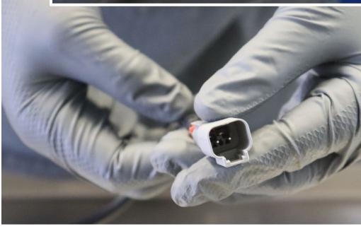
7. After the wire prongs are in place, the green wire locking mechanism needs to be inserted into the plug using a flathead screwdriver. It will be inserted into a slot directly below the wire prong ends that show in the connector body. Be sure to insert this clip correctly.
