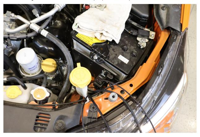
6. Remove the plastic trim piece above the driver side fender by releasing the two plastic clips with a flathead screwdriver as shown. (Flathead Screwdriver)
