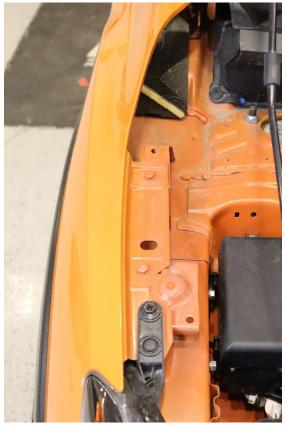
25. Remove the foam insert located in the passenger side gap between the fender and the frame of the vehicle. Route the longer light pod connecting wire across the engine bay and insert the pod wire into the gap. Let it hang freely so there is play when fastening the wire to the harnesses installed in step 7.
