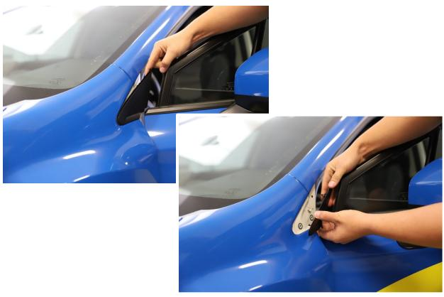
2. Remove 10 MM bolt as shown (10 MM socket) Repeated for both sides.
