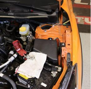
7. Place a provided sticky harness on the fender rail directly right of the battery as well as across the top of the engine bay as shown
