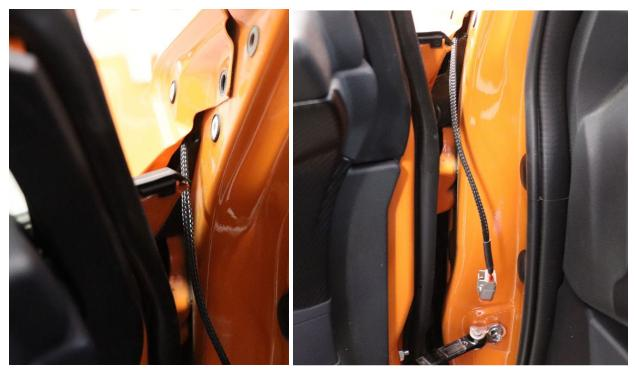
4. Connect the wire ends between the harness and the light pods and feed the excess wire back into the fender well.
