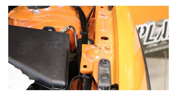
23. Take the switch wire that is running through the firewall and route it so it passes through the first sticky harness on the driver's side. **This wire will only be attached at this sticky harness**. The passenger side pod wire will run through this harness and the remaining harnesses placed down in step 7. **Do not tighten any zip ties at this point.**
