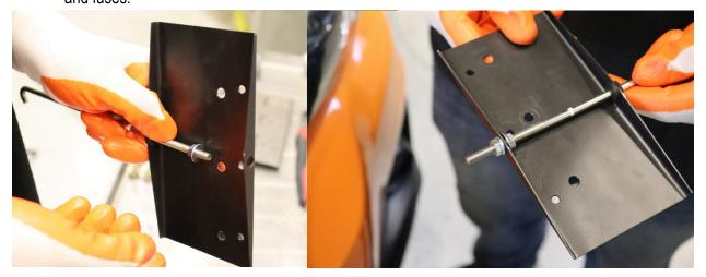
4. Attach the mirror light pod relay to the relay plate. (position on the plate does not matter)
