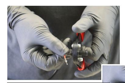
NOTE: Once the wire ends are crimped with the connectors, slide the wire through the lower hole on both of the CDR Series Mirror brackets. This is done so you can mount the pods with the wire in the proper position. The final results are shown below for reference.
