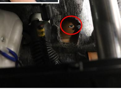
12. Clean out the hole to prepare it to receive the rubber grommet. Once clear of debris, insert the provided grommet
