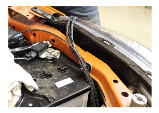
9. Route the wires towards the top of the driver side of the engine bay and set to side.
