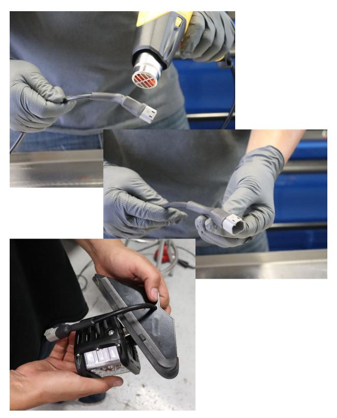
10. This plug is now ready to be connected to the wiring harness detailed in part one of this install sheet
