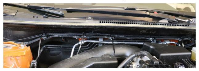
22. Use Zip Ties to bundle the wires leading up from the battery and relay plate together. This will keep the set up clean and ensure the wires run smoothly under the plastic fender trim removed in step 6.
