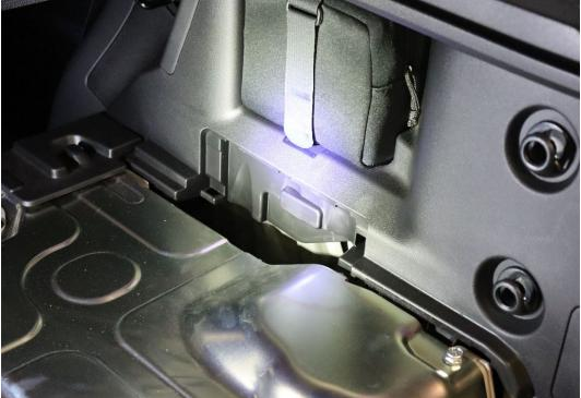
A3. You will see the strut mounting locations down inside these cavities. Use a 14mm Socket and an extension to loosen the top strut mounts. Once this is completed, refer back to step 25 in the body of the installation instructions for guidance.
