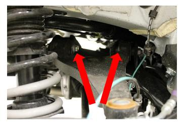
26. Loosen but do not remove the front lower control arm bolts (17mm socket) Repeat for opposite side.
