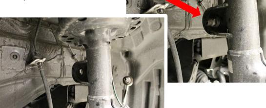
3. Remove the brake line bracket at the strut body (12mm socket). Let hang out of the way. Note how the brake line is run from the underside of the strut body. Installation will be changed in a later step.
