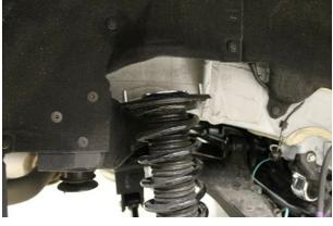
**29.** Locate the Crawford Performance strut extension. Install the short stud extensions provided to top of strut (16mm box wrench). Add thread lock before installing stud extensions. Slide the Crawford lift kit spacers to the strut.
