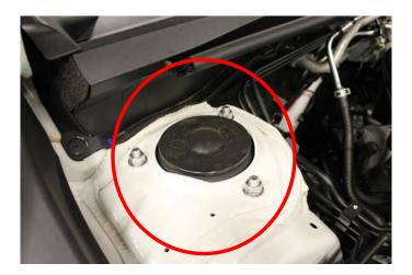
8. Remove factory strut assembly from vehicle
