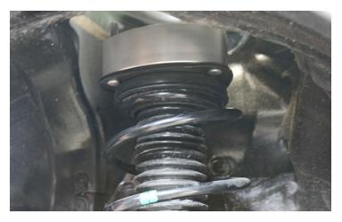
11. Align the three upper strut stud extension threads to the holes on the vehicle and fasten utilizing the provided M10 x 1.25 strut flange nuts. (14mm socket) When installed correctly, the Crawford Performance logo will be legible through the strut tower when facing the engine compartment. (Driver side shown)
