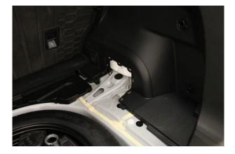
24. Remove the strut nuts and set aside (14mm Socket) Repeat for opposite side.
