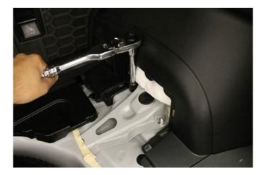
25. Loosen but do not remove the upper control arm bolts (17mm socket). Repeat for opposite side.
