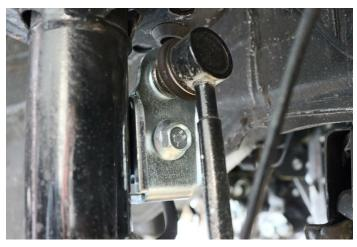
18. Install / Clip factory ABS wire harness onto strut
