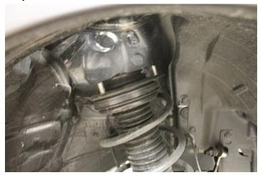
**9.** Locate the Crawford Performance front strut extension. These are universal and fit the passenger and driver side equally. Apply a drop of Loctite to the strut studs, install to the top of the strut using the provided strut extensions (16mm box wrench).
