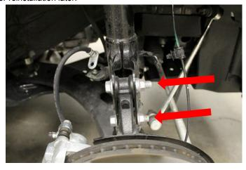
**6.** While keeping the lower control arm supported, release the knuckle from the strut body and let hang out of the way. Make sure to not overextend the ABS, brake line, and CV axle. Adjust as necessary.
