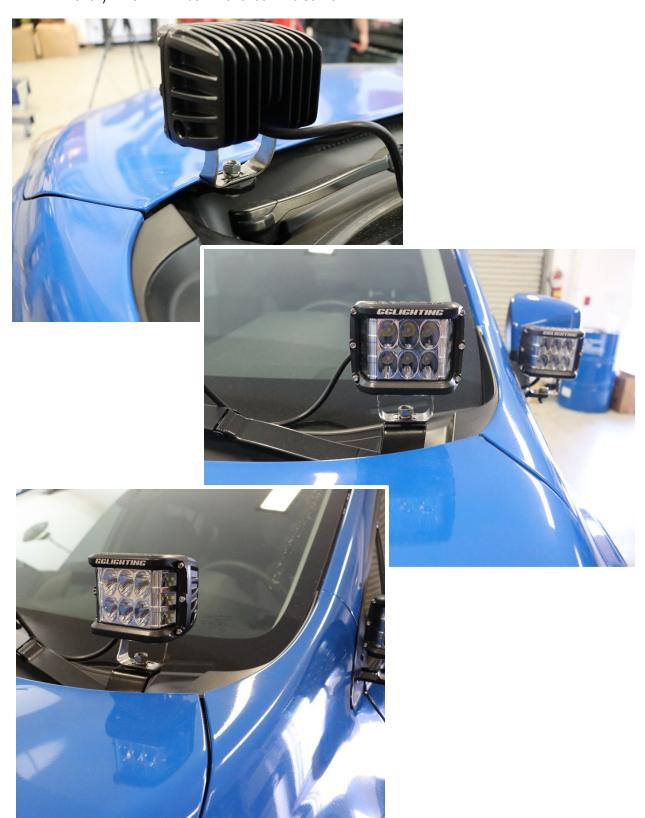
7. Funnel the CDR series pod power supply under hood to be connected to the wiring harness.
