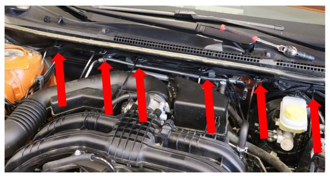
24. Zip tie the pod connector to the hood bracket as shown.
