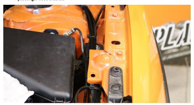
23. Fasten the wire running across the engine bay to the sticky harnesses mentioned in step 7. Fasten the switch wire lead mentioned in step 20 to the designated sticky harness while also running the passenger pod wire through this harness. Make sure to leave enough slack to attach the pod connector to the hood bracket without too much strain.
