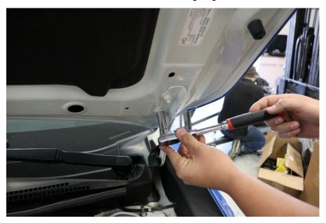
3. Align light pod bracket with hood mount bracket. Fasten to hood with Factory 12 MM nut removed in previous step. The hood bracket nut closest to front of vehicle does not require removal, the light bracket uses this nut to align properly on vehicle.
