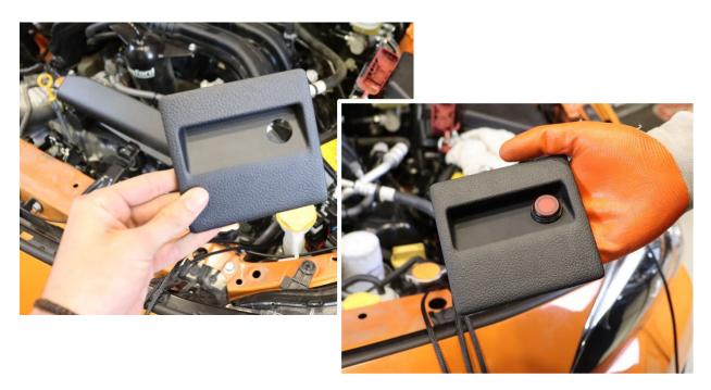
16. Remove the switch from the fuse board cover panel and reinstall the panel into the car. Feed wires from firewall through the panel hole you just drilled out.
