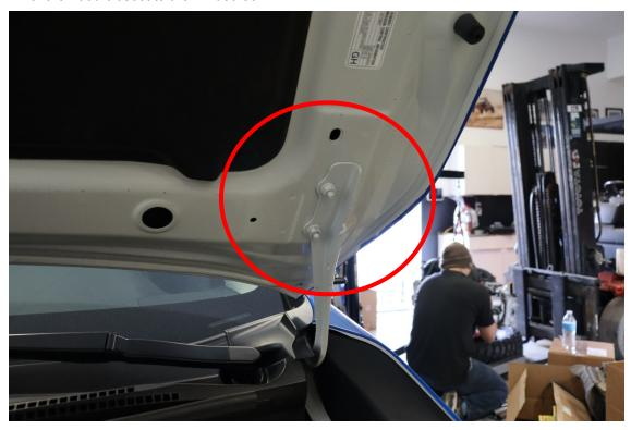
2. Remove lower hood bracket nut on one side of the vehicle (12 MM socket and 3/8" nut driver). **Perform this on one side at a time to avoid misaligning the hood.**
