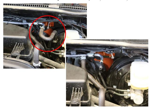
11. Drill a hole through the firewall in the area indicated below.
