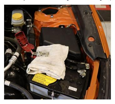
2. Remove the Battery Brace Strut. (10 MM Socket)
