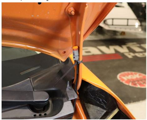
20. Take the switch wire that is running through the firewall and route it through the first sticky harness on the driver's side. **This wire will only be attached at this sticky harness**. The passenger side pod wire will run through this harness and the remaining harnesses placed down in step 7. **Do not tighten any zip ties at this point.**
