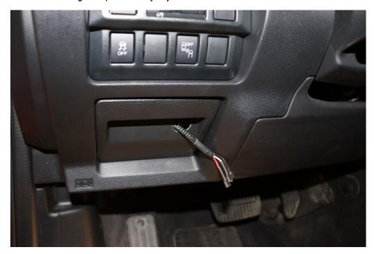
17. Install the wire ends to the switch and re-insert the switch into the fuse board cover.
