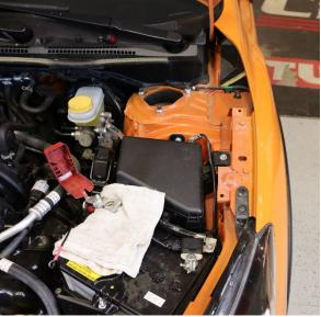
7. Place a provided sticky harness on the fender rail directly right of the battery as well as across the top of the engine bay as shown
