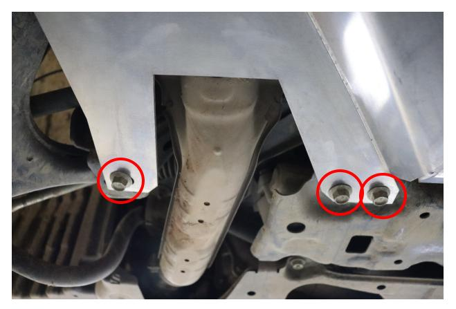
4. Once all the hardware is threaded in place, begin tightening the plate to the sub frame. Torque the bolts to 20 ft-lbs. (14 MM Socket)
