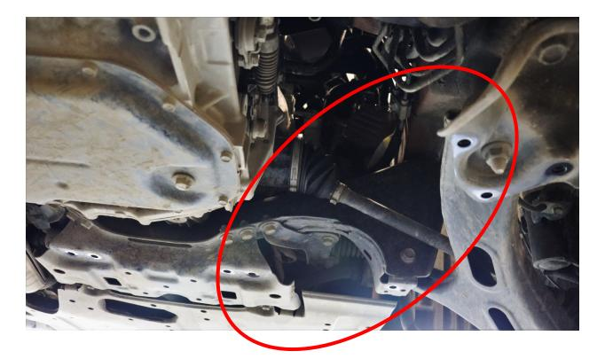
3. Lift the Crawford Transmission plate up into position and loosely thread the provided hardware into the OEM bolt positions that are left open after removing the support struts. This step will be easier with a friend to help hold the plate in place.
