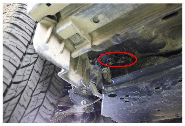
3. Loosely install the front end of the rock sliders (the front of the rock guard will have a cup fitting the bolt slides into) using the OEM 19 MM bolt removed in step one. (19 MM Socket, Ratchet Wrench)
