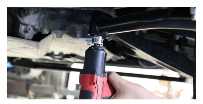
7. Open the doors to the vehicle. Passenger side shown. Your rock guards should be oriented so that the full Crawford Performance Logo is under the front door, while the shortened logo is under the rear door. With the doors open, remove the lowest 12 MM door hinge bolt shown below. (12 MM Socket)
