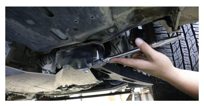
2. Remove the two passenger side rear subframe bolts shown below. (14 MM Socket, Ratchet Wrench)
