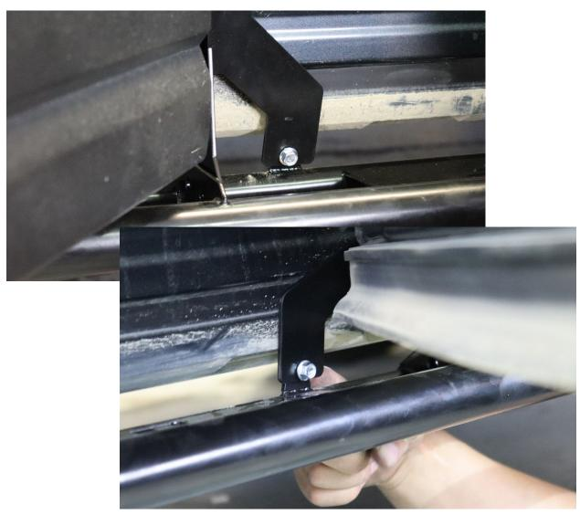
10. Use a floor jack and a rag or other cushion to lift the rock guards into position for the last two 10 MM bolts to be inserted into the center brace mounts. Once raised, fasten the bracket to the rock guards. (10 MM Socket, Ratchet Wrench, 10 MM Box Wrench)
