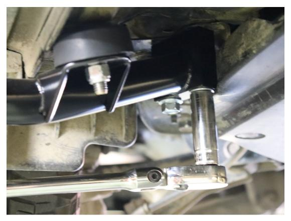
6. Tighten down the front rock guard mount from step 3. (19 MM Socket, Ratchet Wrench)
