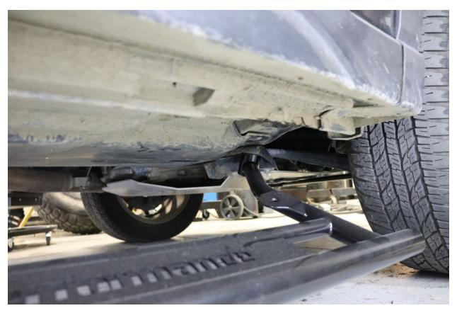
4. Install the rubber sub frame support pads to the tabs indicated below. (9/16" socket)
