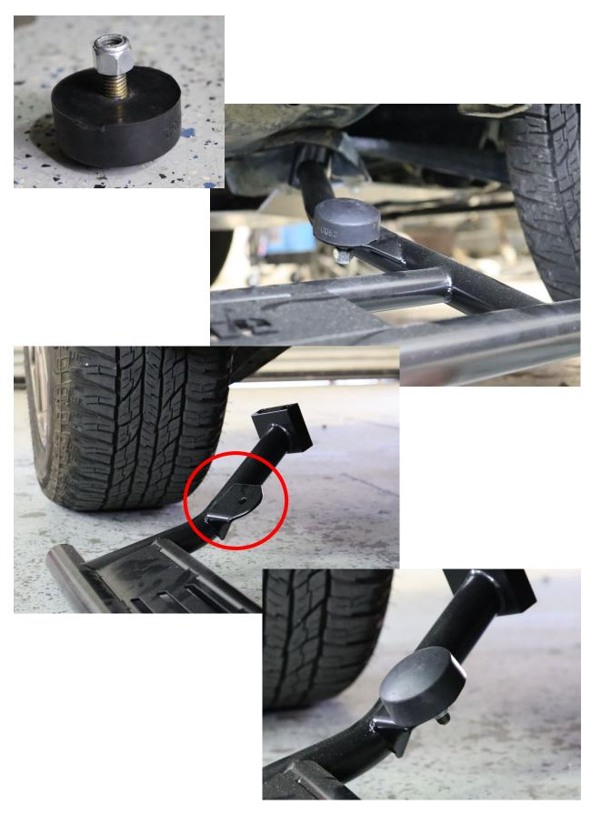
5. Fasten the rear rock guard mount using the provided 14 MM Bolts to the sub frame threads seen in step two. Thread them in by hand before torqueing them down. (14 MM Socket, Ratchet Wrench)
