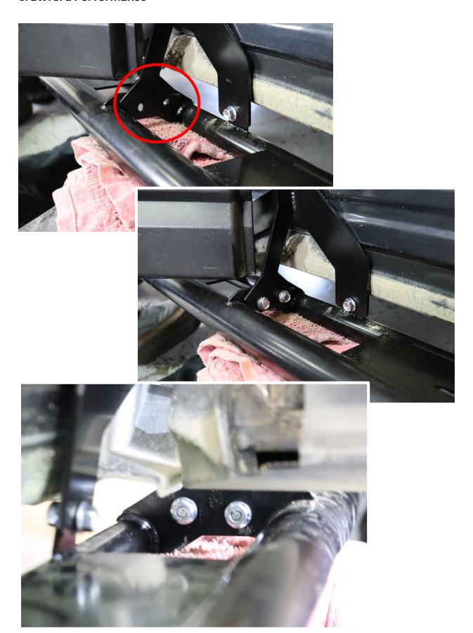
11. Using the floor jack, lift the center of the rock guards under the door frame bracket to align the bracket and the passenger rear door hinge mount. Once aligned, use the OEM 12 MM bolt removed in step 7 to fasten the top of the bracket to the door frame. (12 MM Socket, Ratchet Wrench)
