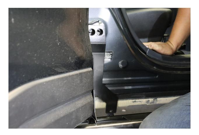
9. Fasten the lower end of the bracket to the rock guards using the provided 10 MM hardware. There are 4 mounting points total to be secured. Fasten the outer tabs before the inner tabs as shown.
