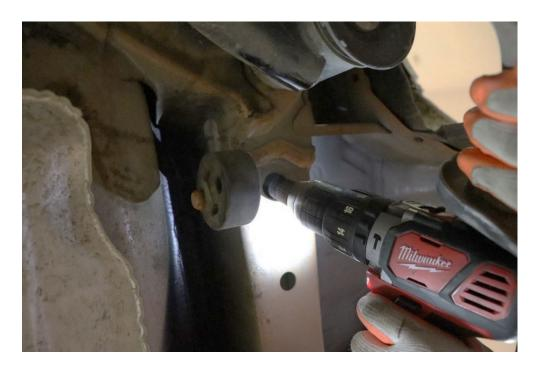
6. Feed the carriage plates into the sub frame through the dremmeled out hole and align carriage plates with sub frame holes as shown. Install supplied fishing wire to the provided carriage bolts.
