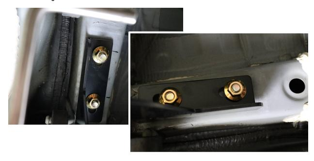
10. Re-secure the exhaust muffler to the hangars, and make final adjustments to bumper positioning
