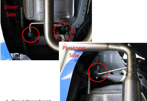
Removal of hanger from midpipe may be necessary to allow for enough play to move exhaust during bumper installation.
