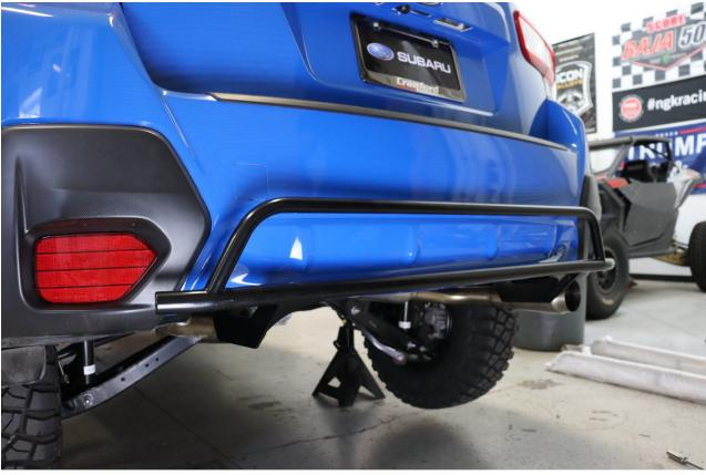
12. Double check all bolts are tight, and that exhaust is reinstalled correctly. Jostle car by the bumper to ensure its secure to the vehicle. We Recommend keeping any OEM parts removed just in case this install needs to be undone.
