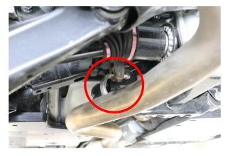
4. Remove plastic grommet from sub frame on both the driver and passenger side so that all six holes are open and accessible.
