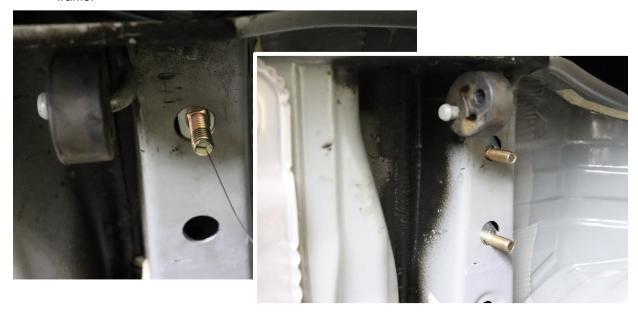
9. Align Bumper mounting tabs with the hanging carriage bolts and secure using provided 19 MM nuts. It may be necessary to have an extra helper to help hold/secure bumper in position. Tighten with fingers to start.
