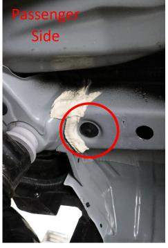
5. Dremel out the holes closest to the front of the vehicle on the passenger and driver side so that the carriage plates and the carriage bolts can be fed into the sub frame rail. Only dremmel out the front most hole on the sub-frame rails.
