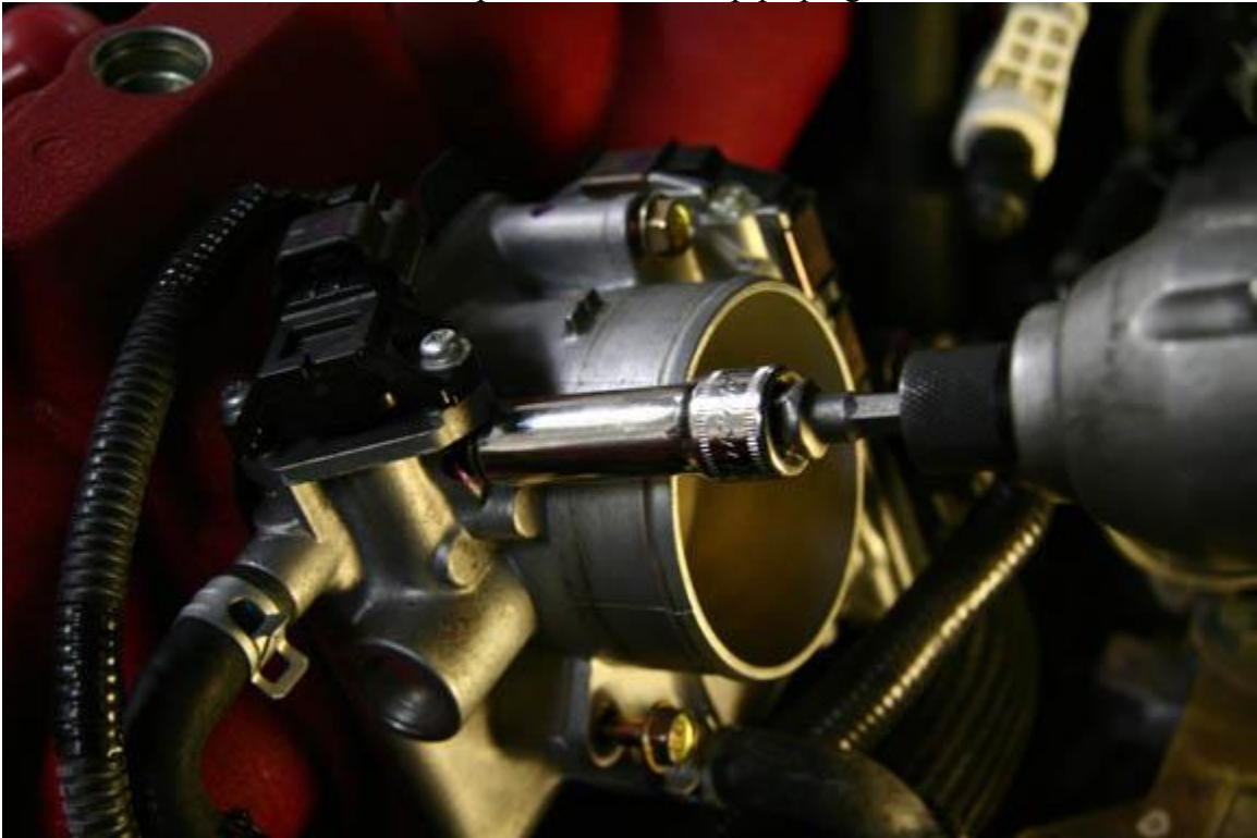
20. Place the throttle body back on the intake manifold (be careful not to harm the throttle body gasket). Screw the four bolts back into the intake manifold and hand tighten.
