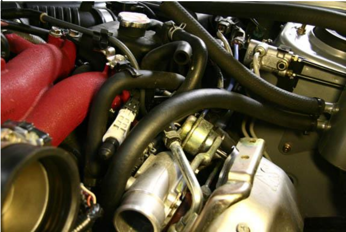
32. Run the second hose from the bottom over the turbo and down to the plastic crank case "Y" connector.
