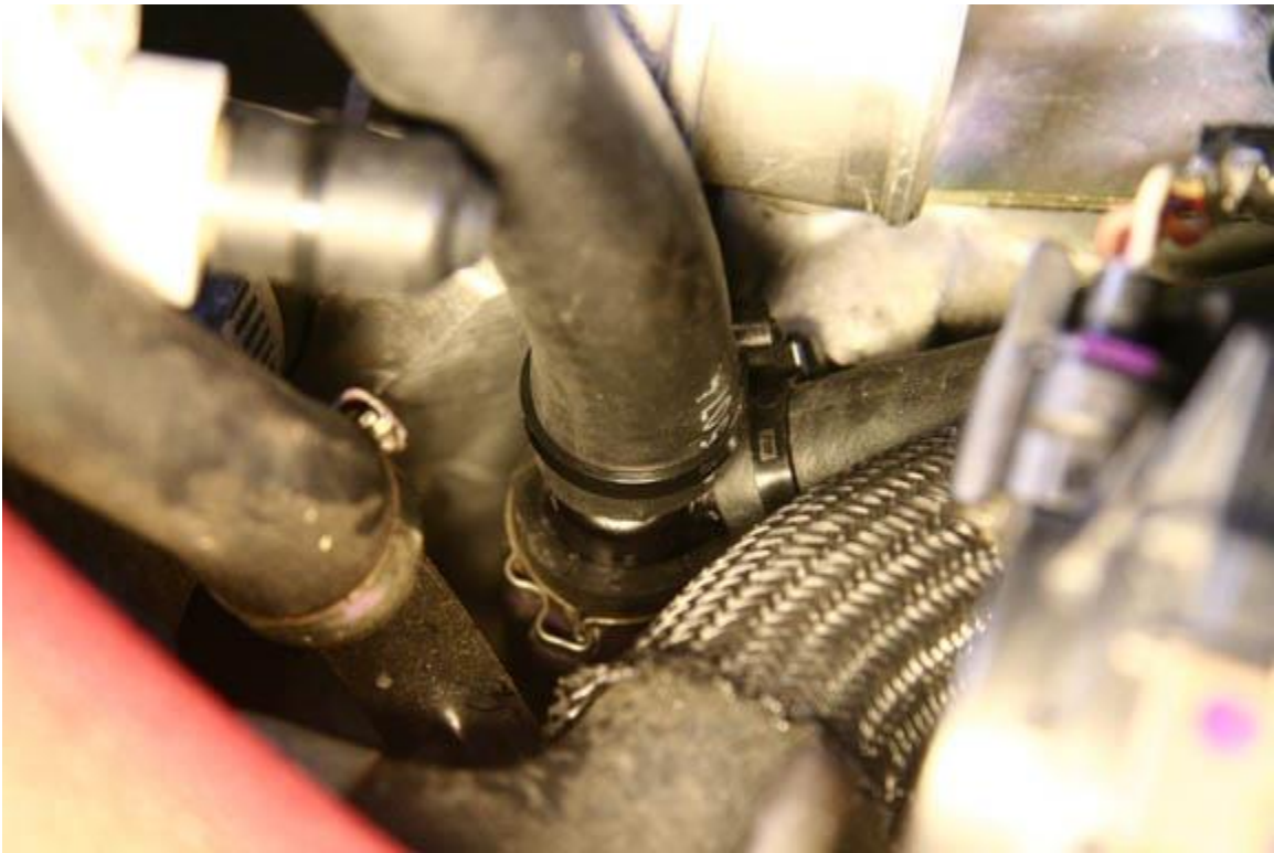
34. Once it is over the plastic “Y connector then use a supplied worm clamp to secure it to the connector. It does not need to be too tight.
