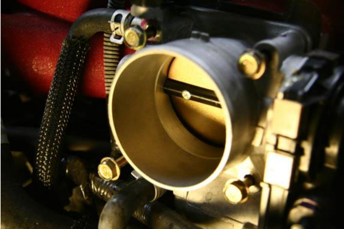
15. Unscrew and remove the 4 bolts holding the throttle body in place.
