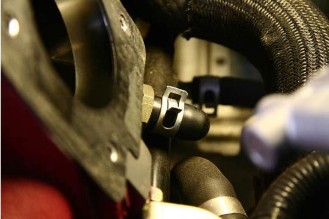
19. Remove the PCV valve and replace with the 1/4" pipe plug.
