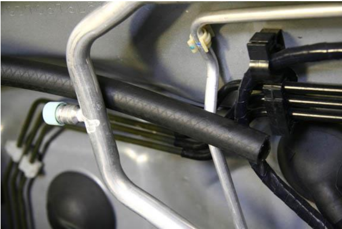
26. Run the longest hose on the Air/Oil Separator around the back of the Air Conditioning line.
