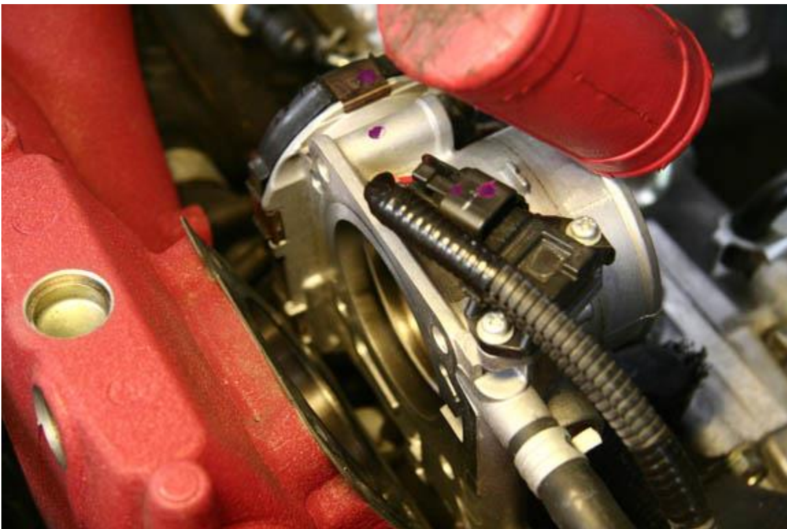
16. Tap the top of the throttle body to break it free from the gasket and intake manifold. Use either a rubber hammer or piece of wood.
