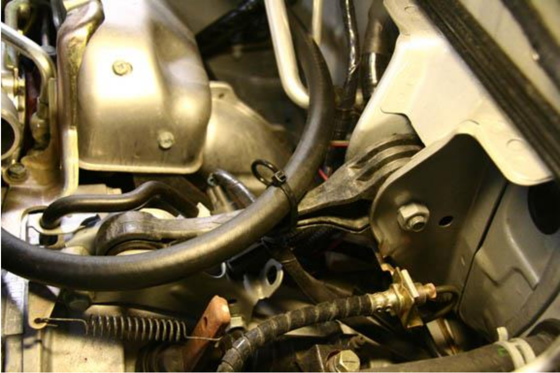
31. Loosely zip tie the bottom hose of the Air/Oil Separator to the pitch stop to hold it in place.
