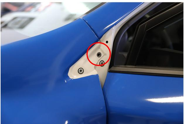
3. Prepare both brackets for mounting by installing the factory weather-strips from the plastic covers removed in step 1 to the Crawford mirror pod bracket. Use the provided double sided tape to reinstall the rubber weather-stripping
