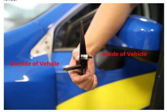
5. Mount bracket on to vehicle. Leave lower hole open for wiring (8 MM allen wrench). Tighten with 8 MM allen wrench and adjust bracket for correct orientation as you tighten
