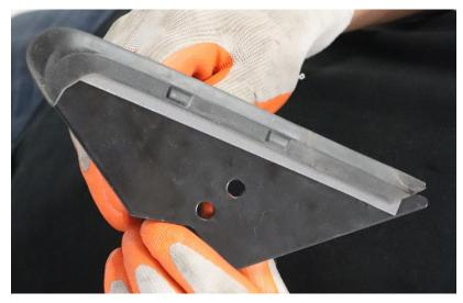
4. Finish bracket prep, by inserting provided button head allen wrench into the upper hole position. Leave the lower hole empty, this will be used to route the pod wire into the car. Slide provided spacer on to allen bolt extruding from the bracket. Spacer should be positioned to the inside of the vehicle.
