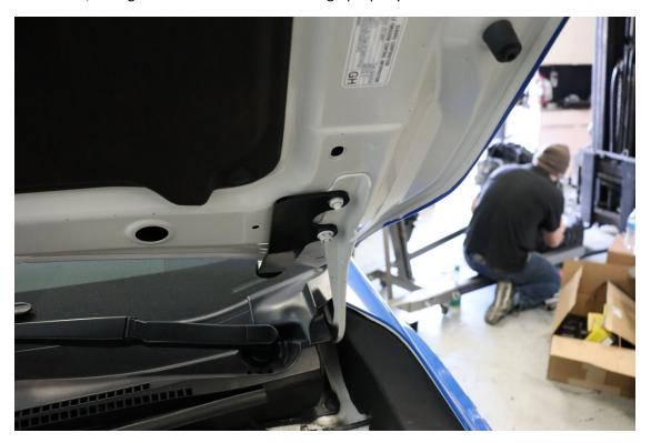
4. Make sure bracket is tightly fastened to the hood. Repeat for the opposite side of the vehicle, making sure to only remove specified fastening hardware.
