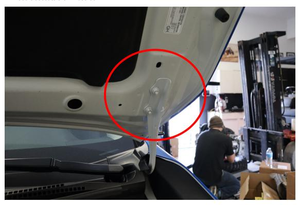
2. Remove lower hood bracket nut on one side of the vehicle (12 MM socket, 3/8" nut driver). **Perform this on one side at a time to avoid misaligning the hood.**
