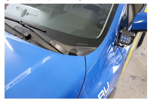
5. Complete set up with desired light pod and wiring set up. Make sure bracket is secured to vehicle.
