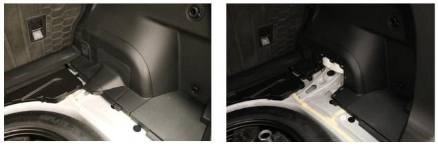
24. Remove the strut nuts and set aside (14mm Socket)
