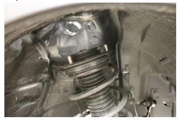
**9.** Locate the Crawford Performance front strut extension. These are universal and fit the passenger and driver side equally. Install to the top of the strut using the provided strut extensions (14mm box wrench).
