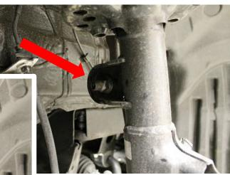
3. Remove the brake line bracket at the strut body (12mm socket). Let hang out of the way. Note how the brake line is run from the underside of the strut body. Installation will be changed in a later step.
