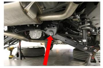
28. Remove both the factory lower rearward control arm bolt at the knuckle and the factory lower strut bolt (17mm socket), then lower the control arm and remove the factory strut assembly from the vehicle Warning: Hold strut assembly while lowering the control arm
