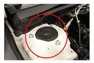
8. Remove factory strut assembly from vehicle
