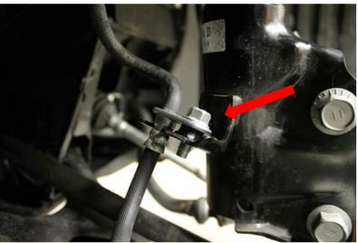
**15.** Install the Crawford Performance sway bar bracket to the strut using the provided M12 bolts, washers, and nuts (14mm socket + 14mm ratchet wrench). Do not tighten at this time. If you have not started the opposite side of the vehicle at this time, you may not be able to line the sway bar up until the opposite side is released.
