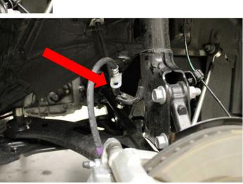
4. Remove the ABS harness clip at the strut body (flathead screwdriver). Let hang out of the way.
