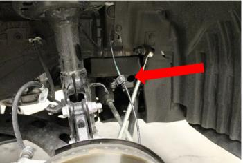
5. Remove the strut to knuckle bolts. The bolts are specific to upper and lower mounting locations and direction of install (19mm socket + 19mm ratchet wrench). The upper is a cam bolt, while the lower is a standard bolt. Make sure to note their orientation for reinstallation later.
