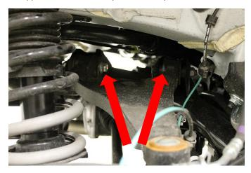
26. Loosen but do not remove the front lower control arm bolts (17mm socket)
