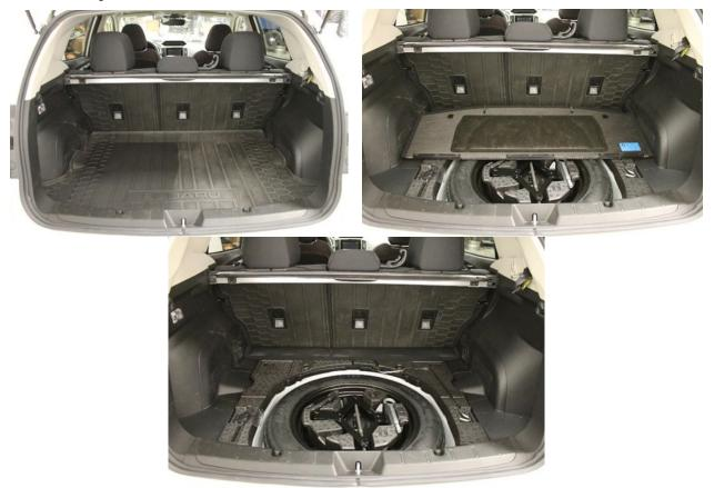
**22.** Remove the 4 clips holding the foam support liners, then remove the foam
