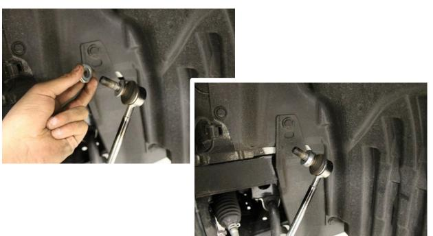
17. Install the factory end link to the Crawford Performance bracket using the factory hardware (17mm socket). Torque the bracket and end link to 45 ft- lbs.
