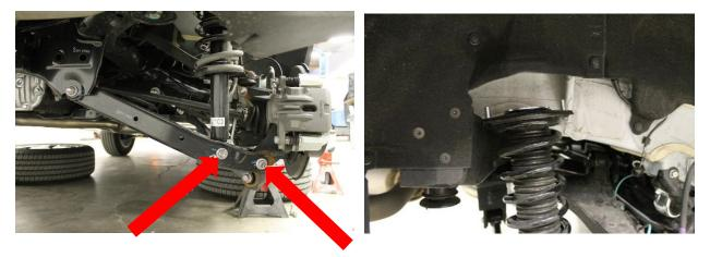
**29.** Locate the Crawford Performance strut extension. Install the short stud extensions provided to top of strut (14mm box wrench). Add thread lock before installing stud extender
