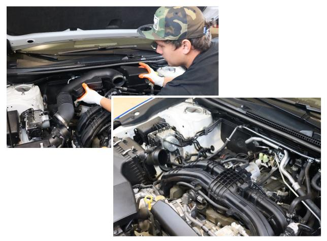
2. Remove PCV hose leading from top of block to the manifold
