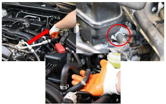
b. Remove clip from manifold tab (flathead screwdriver)
