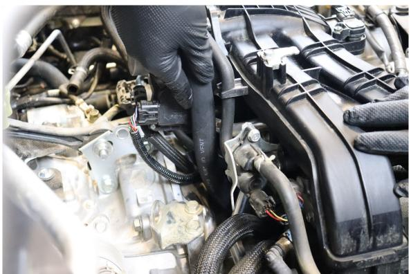
4. Install 13" length of PCV hose on to PCV port on the engine block and route it under the passenger side intake manifold to the front of the intake manifold
