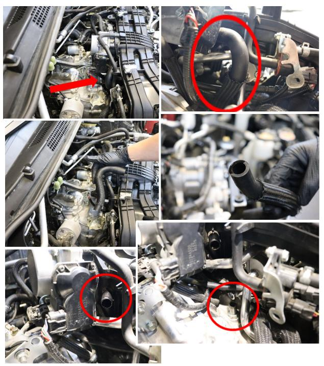
3. Lube the 13" inch length of PCV hose to prep to install on PCV port on block
