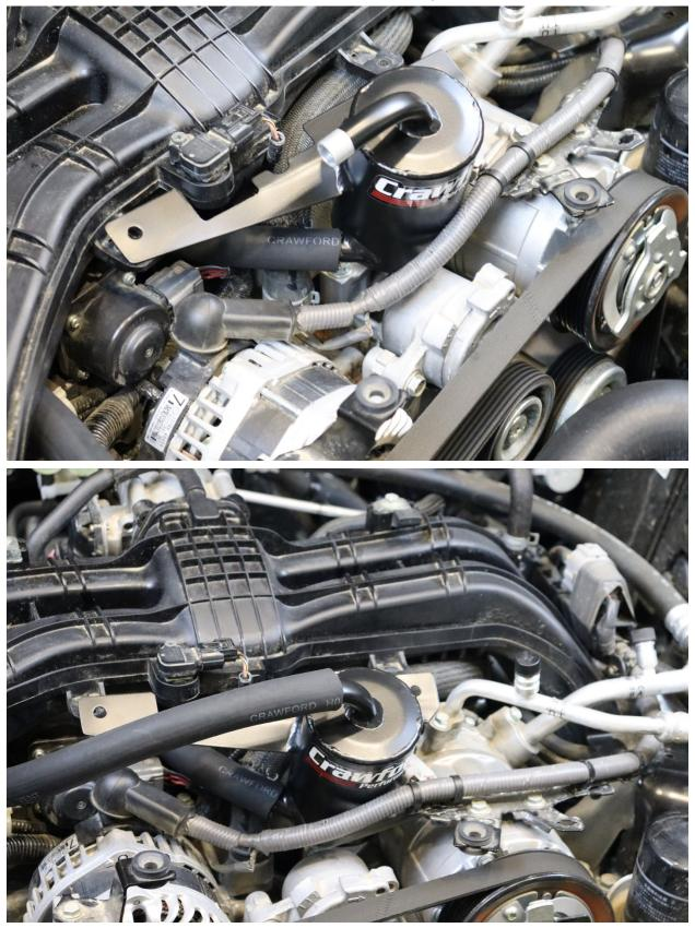
9. Mount the AOS to the front of the manifold using the OEM tabs and provided 10 MM nuts + bolts. Make sure the AOS and all hoses are secured to vehicle. (10 MM Socket, 10 MM Ratchet Wrench)
