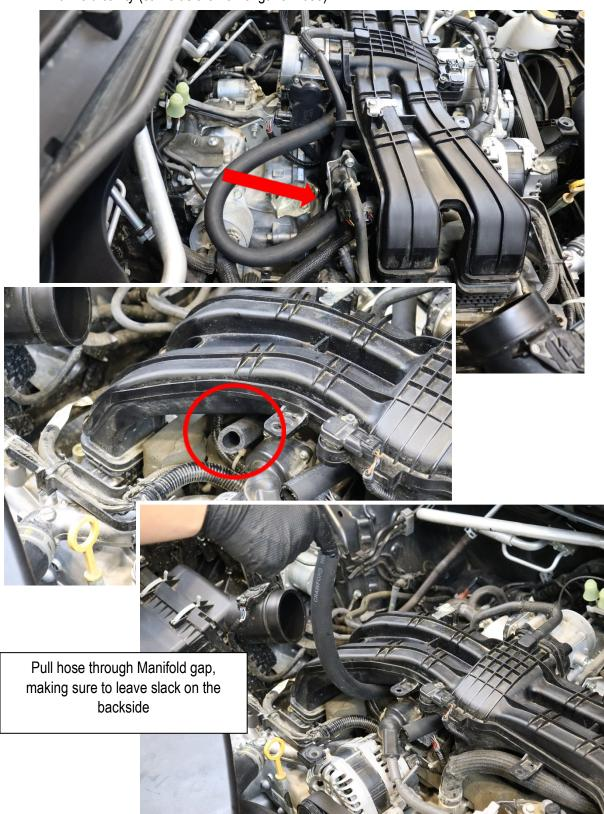
7. Route the 25" length of PCV hose to the front of the intake manifold by going underneath the manifold cavity (same as the 13" length of hose)
