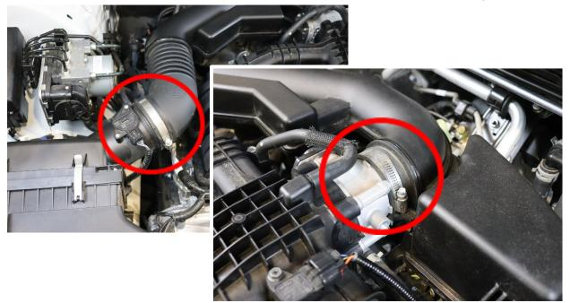
d. Lift off the entire intake assembly and set aside
