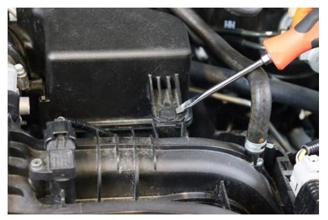
c. Use a flathead screwdriver or 8 MMM Nut Driver to loosen the 2 hose clamps
