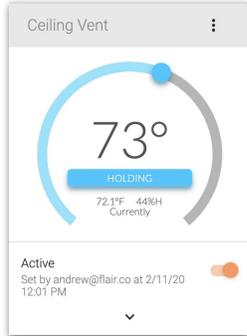
A room tile displays the set point and room temperature for a room. Drag the blue dot to adjust the room’s set point. This creates a room “hold”. Click the blue “Holding” button to set hold options. The default hold duration is set in Home Settings->System Settings. Toggle the “Active” switch to set the room to Inactive. Flair follows “Away Settings” for inactive rooms. Tap the arrow to view Puck and Smart Vent status. Tap the 3-dot menu, then select “Stats” to view helpful room statistics.
