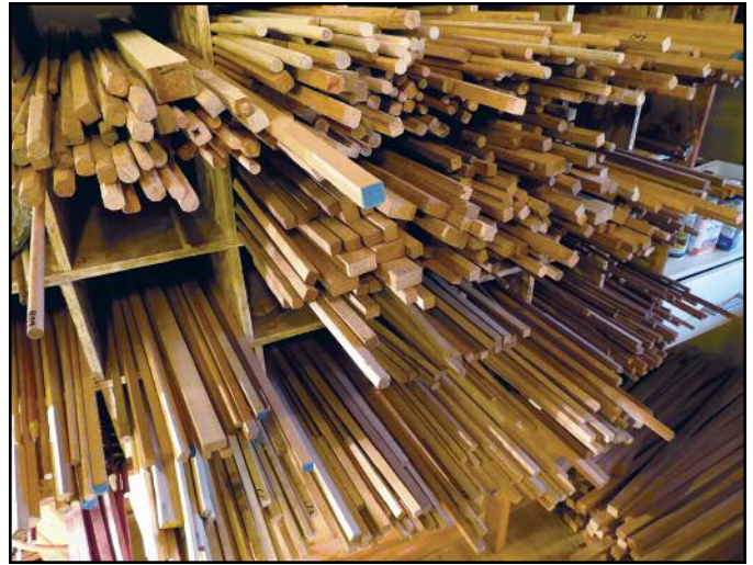
A rack with a wide selection of square shafting billets, dowels, and partially turned shafting.
