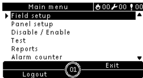
Figure 18: The installer level Main menu
