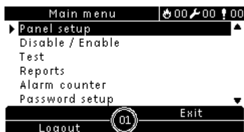
Figure 20: Maintenance level Main menu
